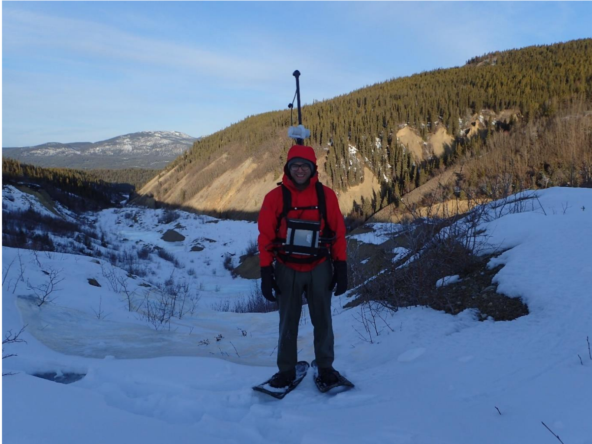
Magnetometer Survey – Livingstone Creek – photo taken March 25, 2016 --The rover magnetometer is strapped to the operator's chest and the sensor coil is above his head. The GPS antenna is attached at the top of the apparatus.
