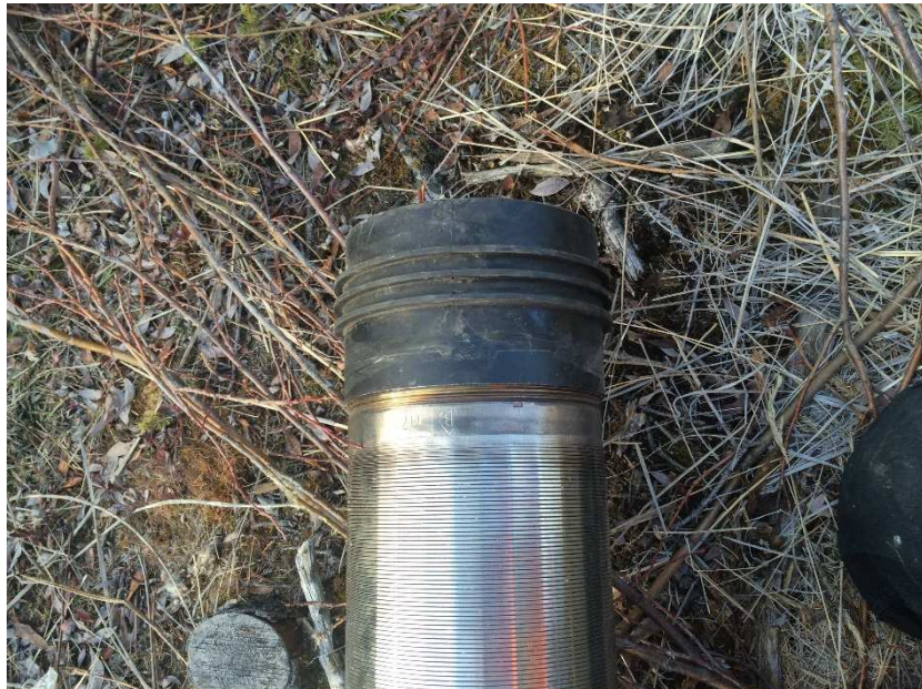
Photo 2: K-Packer and top of 18-slot screen/riser (male thread) prior to installation in KFN-N
