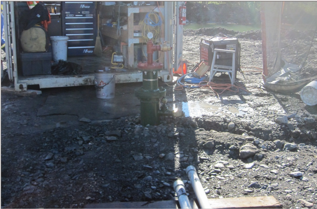
Photo 4: KFN-L wellhead after final pumping test. Note the two valves and pressure gauges. August 23, 2012.
