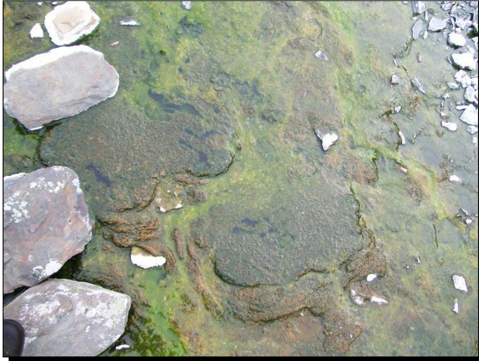
Photo M12 - Algae and iron hydroxide precipitate down drainage ~7m from M08S-6 (September 9, 2008)
