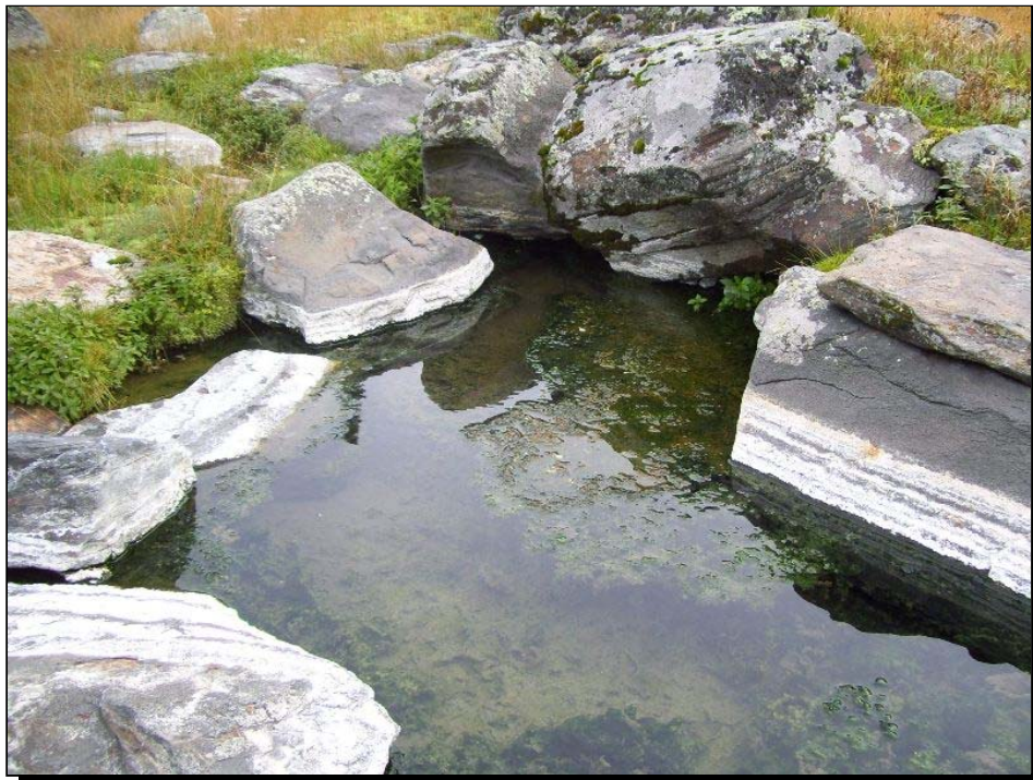
Photo M11 - M08S-6; Likely major vent along with M08S-2 vent. Discharge estimated 20 gpm. White encrusting 10 cm above water level. (September 9, 2008)
