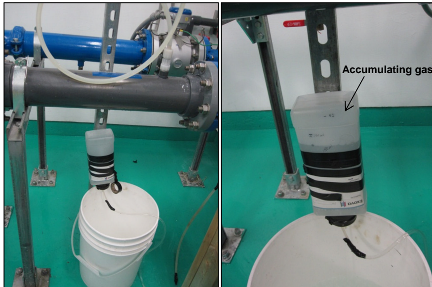
Figure 2: Photographs of the gas trap used to collect a gas sample from degassing well water. (December 5, 2012)
