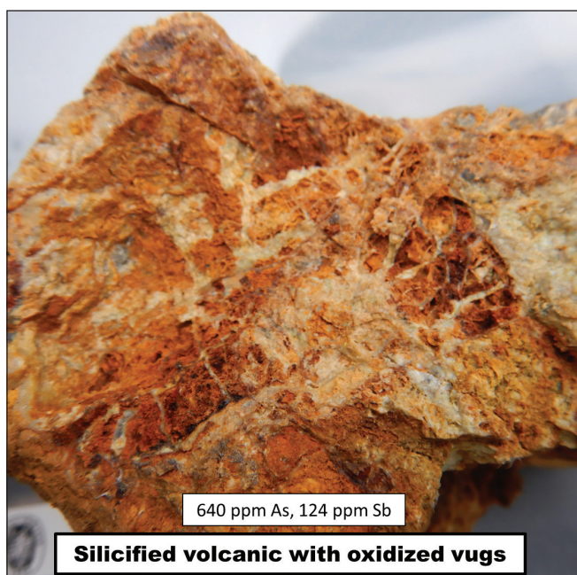
Figure 13. Grab sample of silicified volcanic rock that assayed 640 ppm As and 124 ppm Sb.
