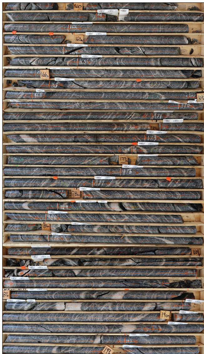
Figure 7. Moderate to high-density, quartz-sulphide sheeted veins at Snowline Gold’s Rogue property Valley target as seen in drillhole V-23-034 from 158.7 to 194.5 m; average grade of this section is 4.32 g/t Au (Snowline Gold Corp., 2023e).
