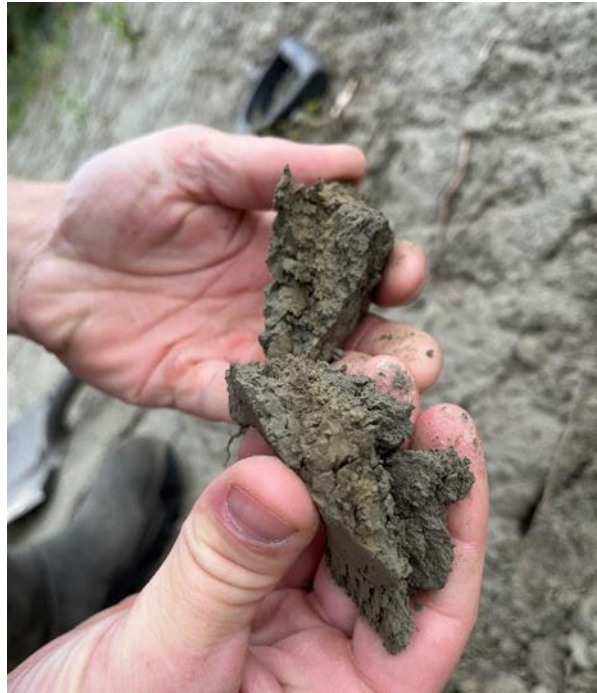
Photograph 6. Low soil constraint, clay-rich material.
