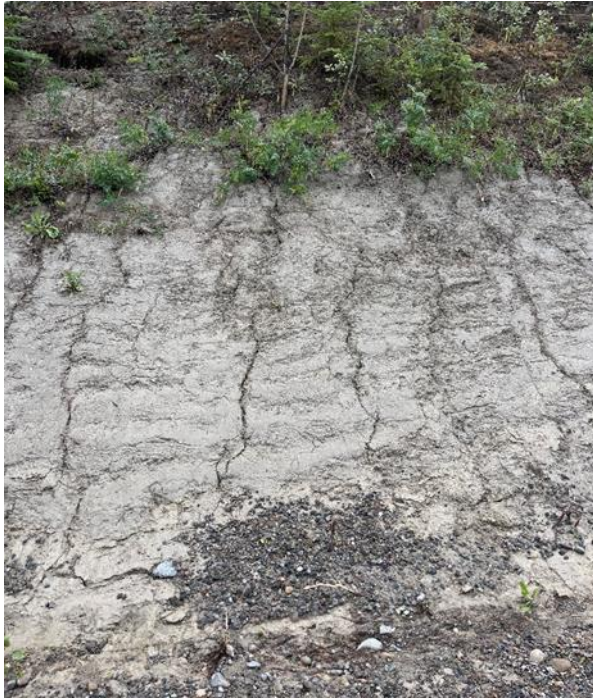
Photograph 5. Low soil constraint, clay-rich material.
