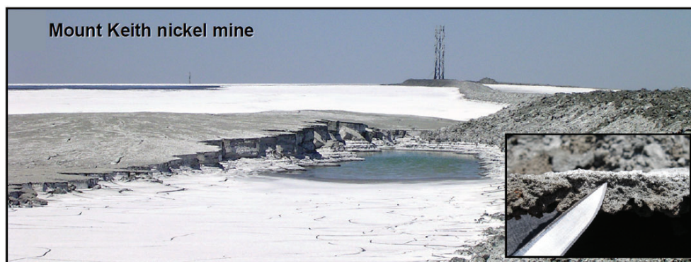
Figure 4. Mineral carbonates forming on serpentinized ultramafic rock tailings at the Mount Keith nickel mine in Western Australia. Image from Power et al. (2014).
