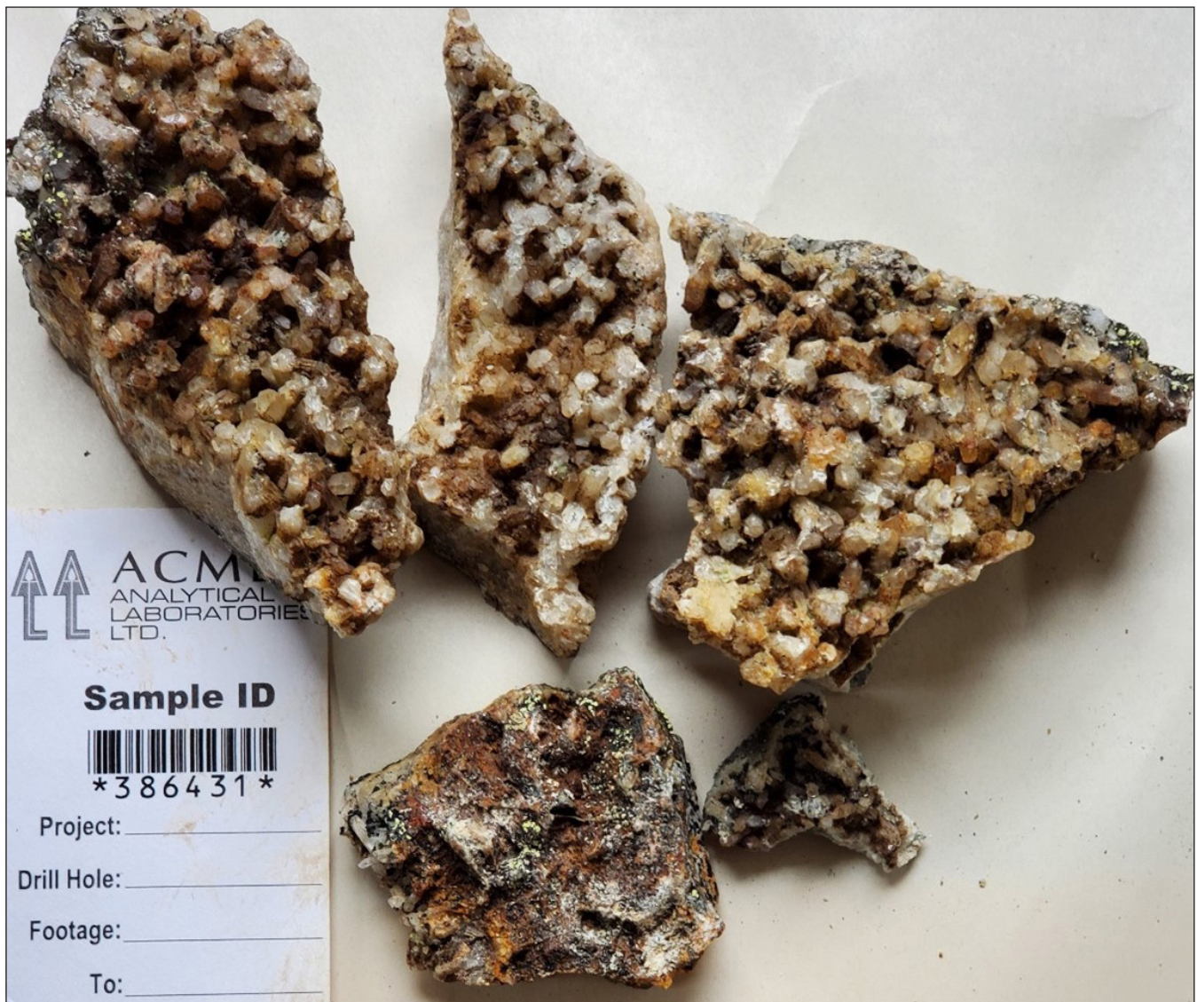
Figure 24. Sample 386431 from the ORC property, containing a drusy quartz vein that ran over Pb and Ag detection limits. Assay tag measures 10 cm in the long direction.
