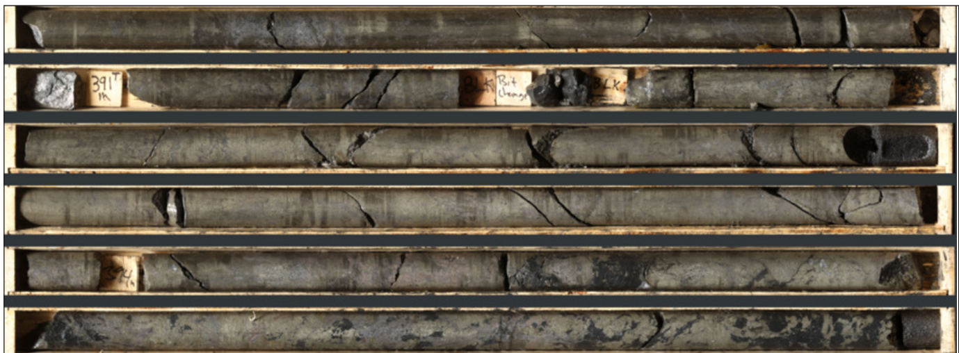
Figure 19. Galena and sphalerite-rich massive sulphides in drillhole NB24-024; 389.9 to 396.0 m at Boundary Zone (Figure provided by Fireweed Metals Ltd. [Fireweed Metals Ltd., 2024c].)
