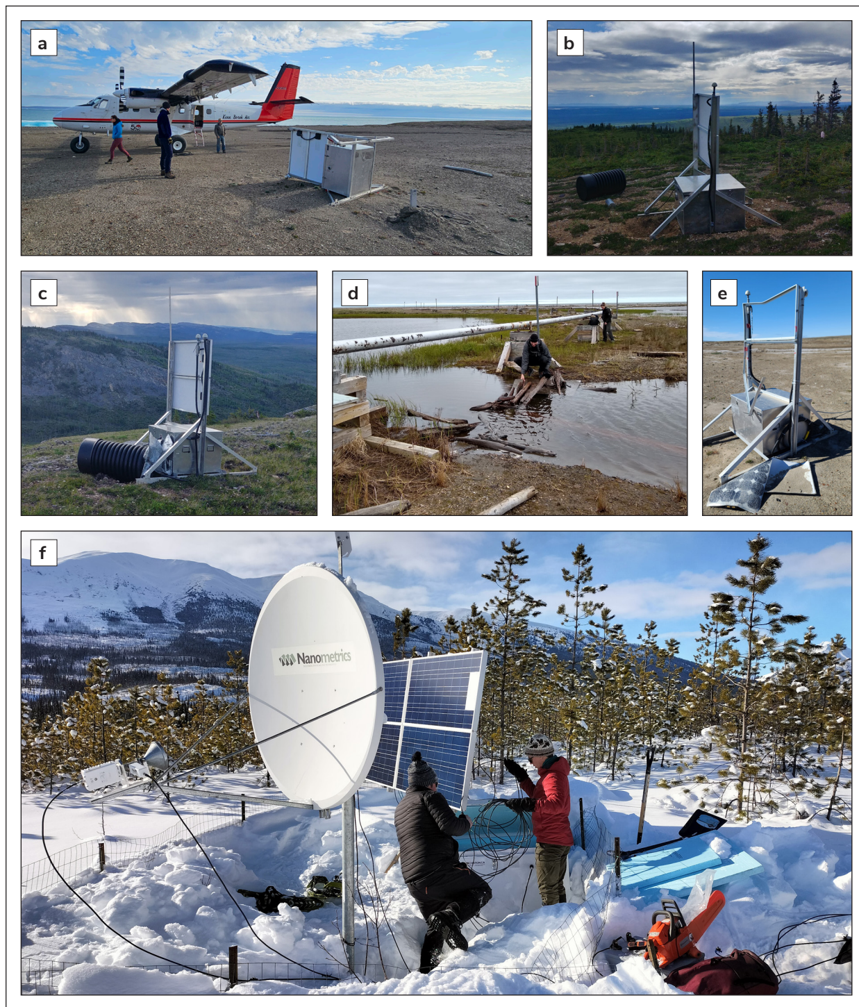
Figure 6. Common challenges encountered operating geophysical instrumentation in the Canadian north. (a) Site access requires a chartered aircraft capable of off-strip landing. Also pictured is common damage to instrumentation, where polar bears have knocked over the 400 lb. battery and electronics kiosk with mounted solar panels. (b, c) Examples of helicopter-access-only locations where wildlife, likely grizzly bears, have exhumed the seismometer vault (and sensor). (d) Unexpected hazards or washouts are not uncommon when visiting remote sites. (e) The winds in some regions can reach hurricane-force speeds, and cause equipment to fail. Pictured here are two solar panels where high winds blew the panel interiors out of their frames. (f) Snow accumulation can present challenges in mountainous regions of the Northwest Territories and the Yukon. In this example, near Nahanni National Park during March, snow removal was required for site access and to expose the solar panels.
