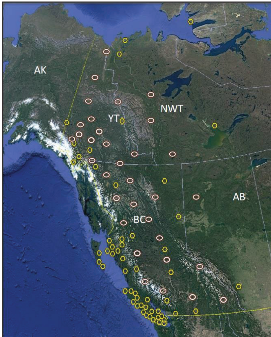
Figure 1: Proposed distribution of seismometers for the CCArray (courtesy of S. Azevedo and B. Busby). The smaller light blue dots provide a schematic representation of a 165 broadband seismometer array at an 85km grid spacing. The larger red circles are current and planned USArray Transportable Array Stations; other symbols denote existing broadband seismometers installed by other groups. Ocean bottom seismometers would also be deployed in the Beaufort Sea and off the west coast of British Columbia.
