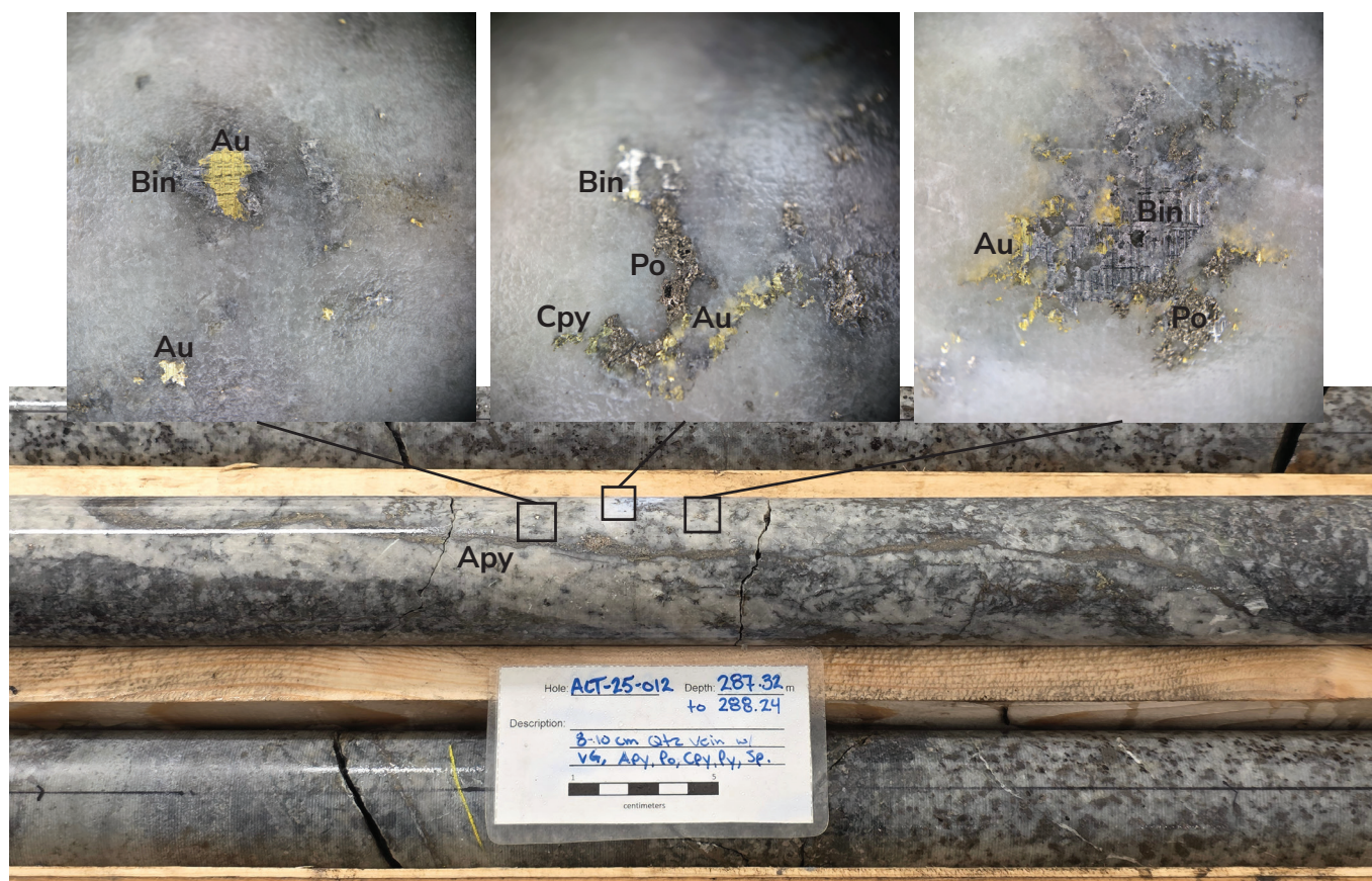
Figure 18. Forge Resources Corp.'s Alotta project drill core showing a ~10 cm-wide quartz vein cutting granodiorite and containing coarse native gold (Au), bismuthinite (Bin), pyrrhotite (Po), chalcopyrite (Cpy) and arsenopyrite (Apy) in hole ALT-25-012. Pyrite, molybdenite and sphalerite also occur, but are not visible in this figure (Forge Resources Corp., 2025b).
