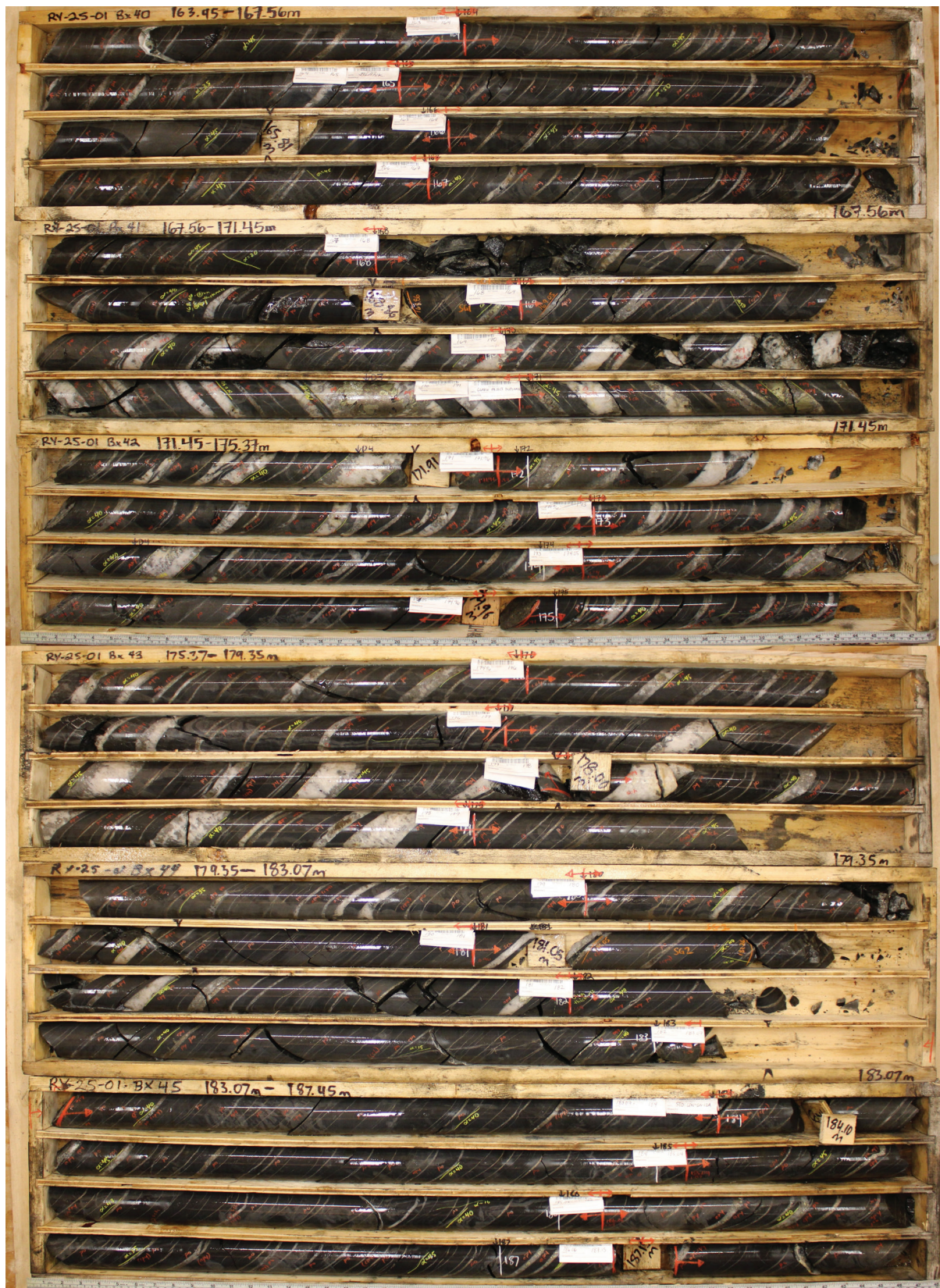
Figure 14. Drill core from hole RY-25-01 at Trifecta Gold Ltd.'s Rye property; sheeted vein density is greater than 25 per metre and consists of quartz-pyrrhotite-chalcopyrite ± arsenopyrite ± scheelite (Trifecta Gold Ltd., 2025a).
