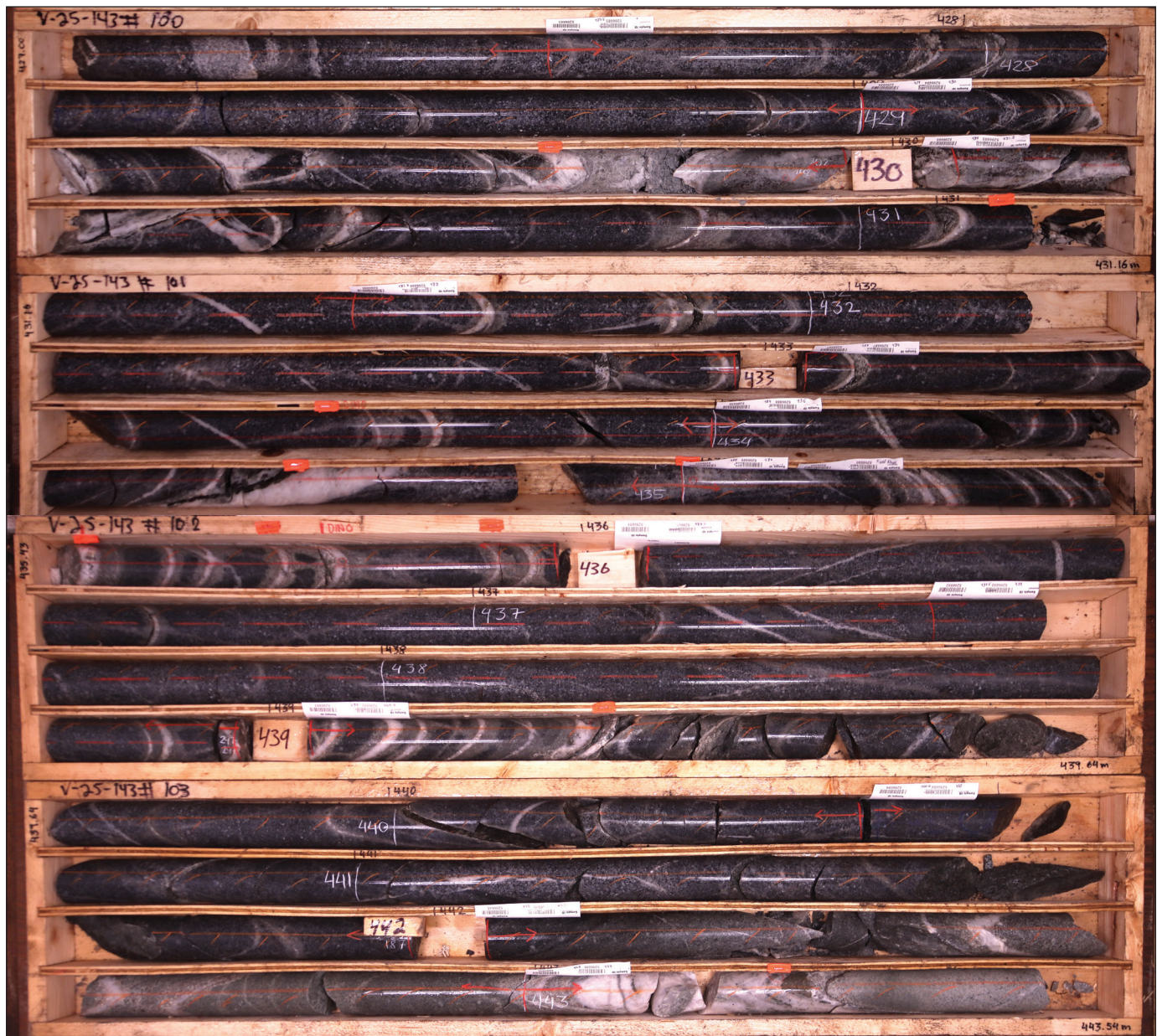
Figure 13. Photos of drill core from hole V-25-143. The interval shown is from 427.0 m to 443.5 m downhole and highlights light to intense sheeted quartz veins cutting the Valley intrusion. These sheeted quartz veins occur along the eastern edge of the Valley intrusion, which was previously assumed to be unmineralized (Snowline Gold Corp., 2025b).
