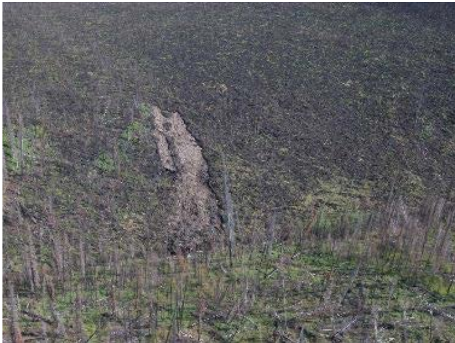
Figure 3. Northwest-facing detachment developed within silt-rich colluvium. This slide is 63 m long and 19 m wide and initiated on a 19 degree slope (05PL012).
