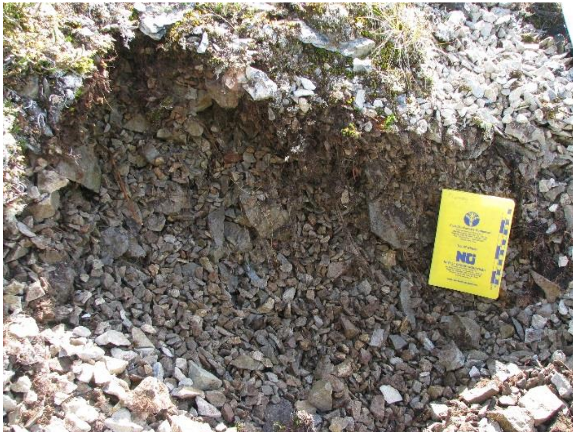
Figure 2. A 60 cm deep pit in the front of a solifluction lobe at the toe of the slope reveals mostly loose cobble and pebble-sized angular rubble with very little fine material.
