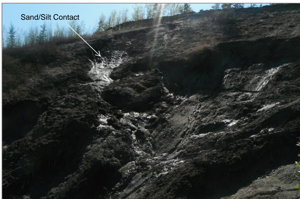
Photo 3: Sand/Silt contact (May 15, 2014)
