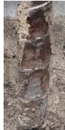
Organics (Unit #2) over Fluvial silt (Unit #3)
