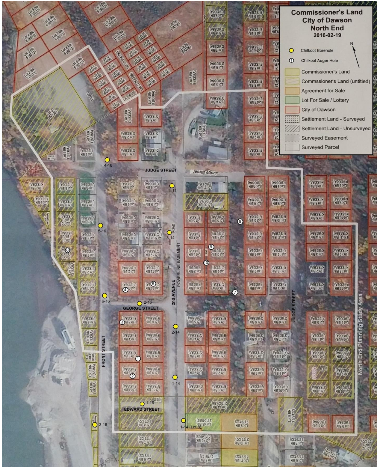
Figure 2 Study Area, Borehole and Hand Auger Locations
