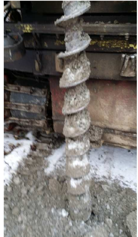
Photo # 3 (above) – BH 4-14 Ice lens @ 4.9 meters
