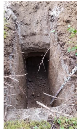
Test pit TP 3-19 soil conditions.
