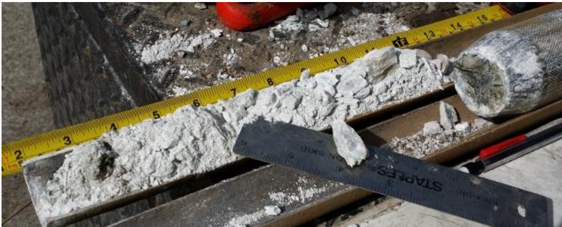
BH 4-16 – Sample No.34 – Unit # 5b Colluvial Slide Debris
