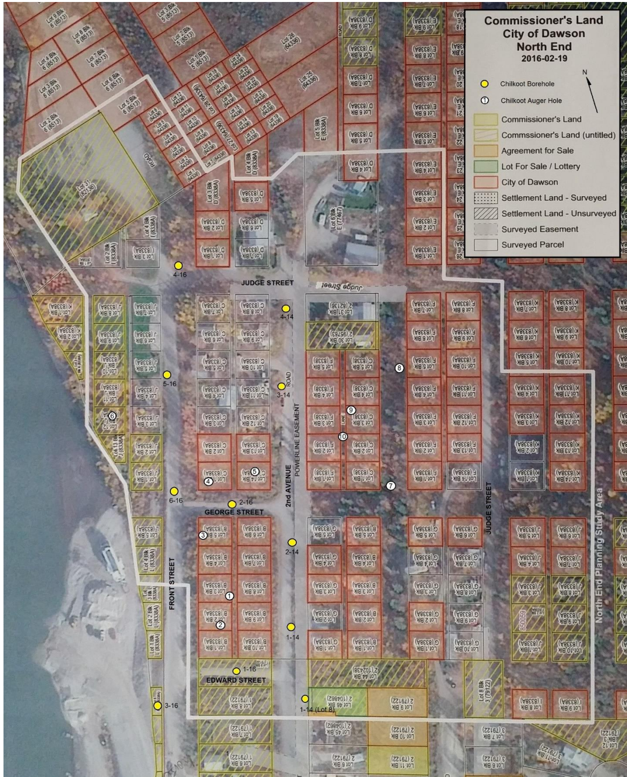
Figure 2 Study Area, Borehole and Hand Auger Locations
