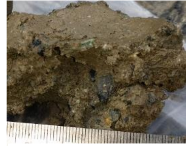
BH 5-16 – Sample No.42 Remnants of Colluvial Apron Deposits
