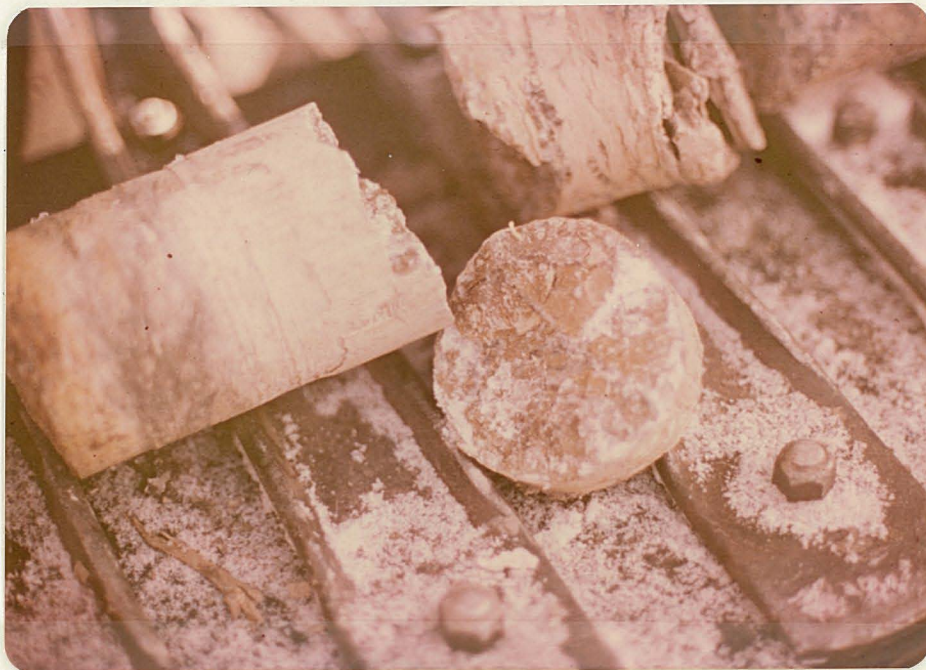
7. The ice lenses are clearly visible in the core sample at 1023+00.
