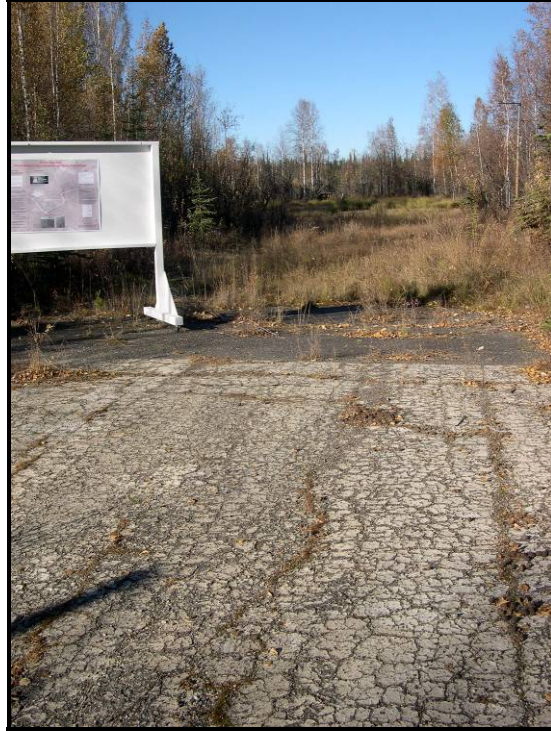
Figure 4-3: Reflective surface test section after 30 years at the CRREL, Farmer's Loop experimental site, Fairbanks, Alaska
