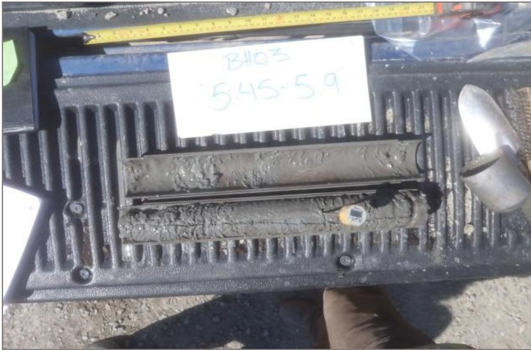
Photo 5: Ice rich SILT in BH03 (5.45 m – 5.9 m)
