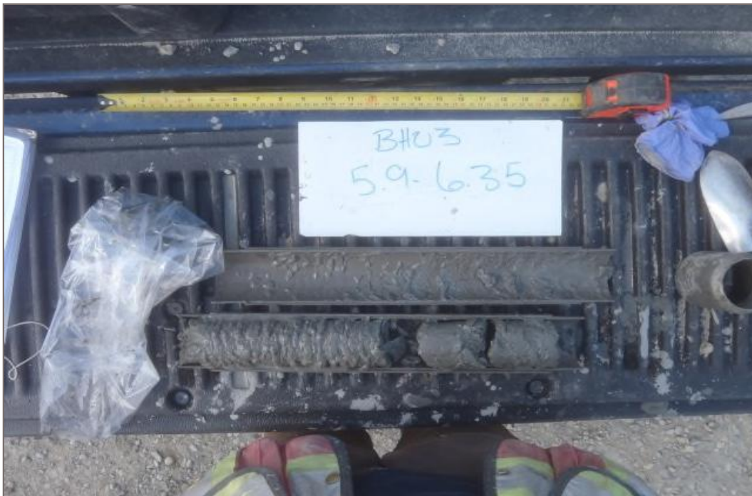
Photo 6: ICE and SILT in BH03 (5.9 m – 6.35 m)
