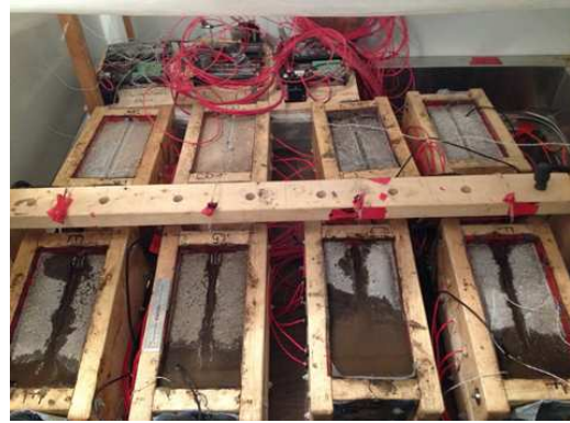
Figure 1. Eight thawing-cells during an experiment in a temperature-controlled environmental simulator.
