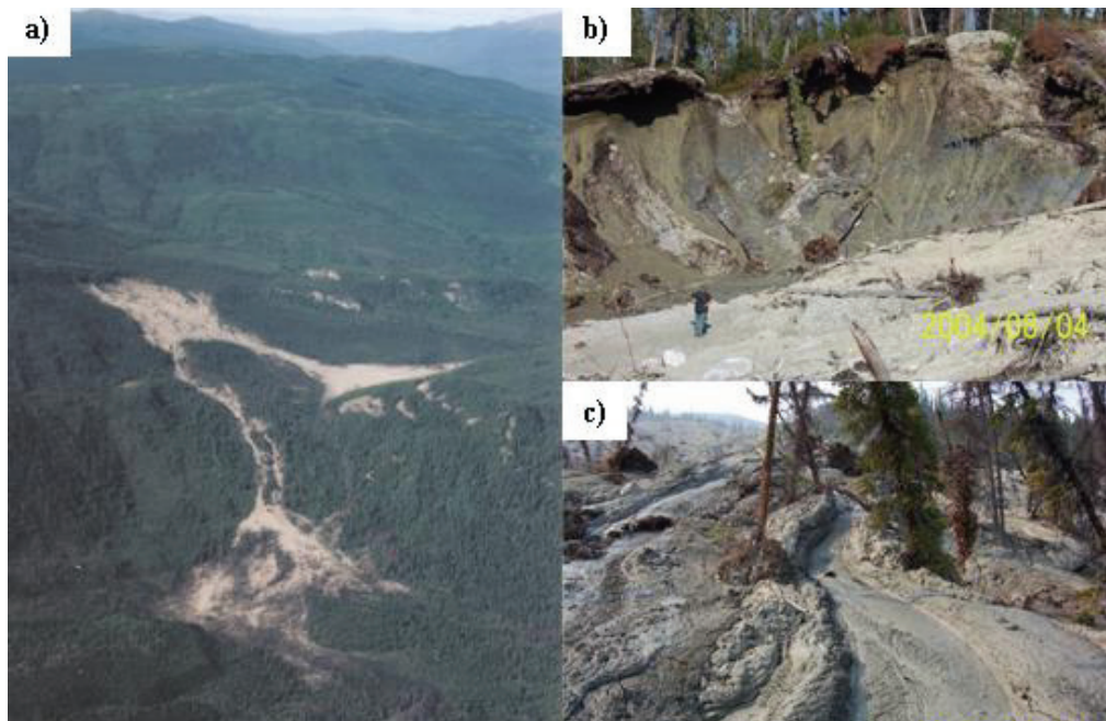
Figure 4: Magundy River Landslide: a) overview looking south (top scarp is 350 m wide, elevation change from top scarp to depositional is about 350 m) b) active thaw slump area (note 2 nd author for scale); and c) active debris flow (channel width is approximately 1 m across).
