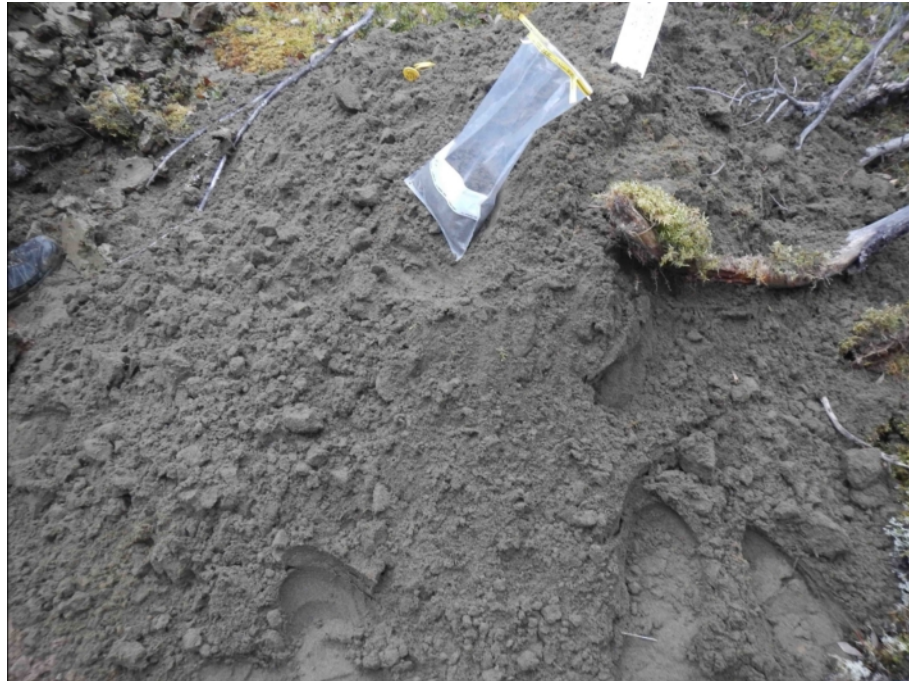
Figure 869-5335.1 Photo of Sample pile from 0.2m to 1.0m below ground level, from Test Pit 5335
