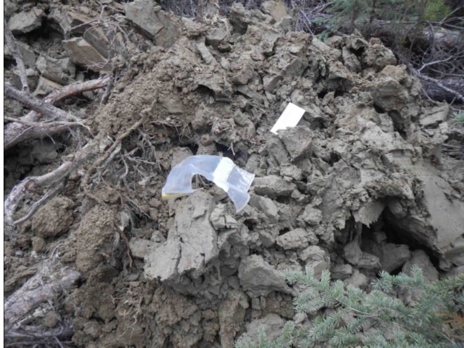
Figure 869-5333.3 Photo of Sample pile from 2.5m to 3.5m below ground level, from Test Pit 5333
