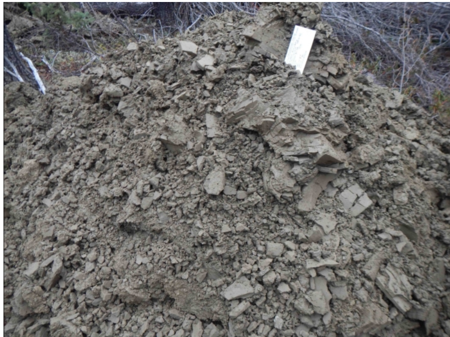
Figure 869-5333.2 Photo of Sample pile from 1.0m to 2.5m below ground level, from Test Pit 5333
