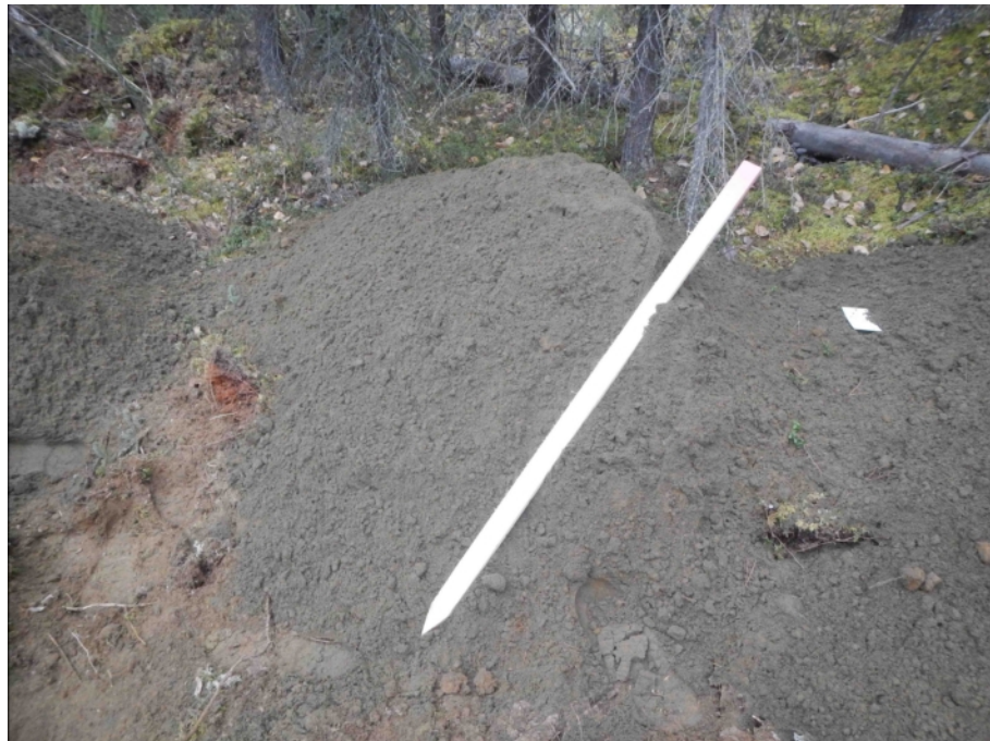
Figure 869-5329.2 Photo of Sample pile from 1.0m to 2.0m below ground level, from Test Pit 5329
