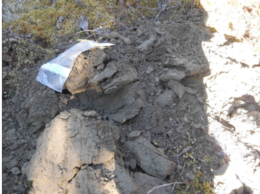
Figure 869-5326.1 Photo of Sample pile from 0.2m to 1.0m below ground level, from Test Pit 5326
