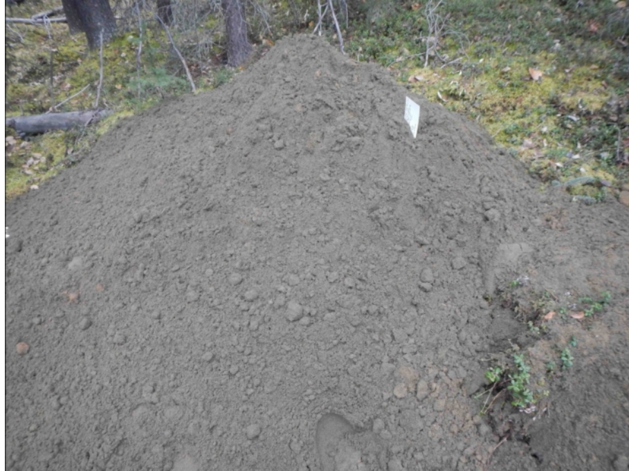
Figure 869-5329.1 Photo of Sample pile from 0.2m to 1.0m below ground level, from Test Pit 5329
