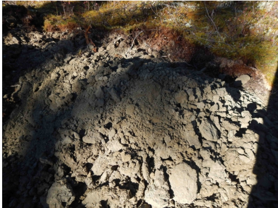
Figure 869-5322.3 Photo of Sample pile from 2.0m to 3.0m below ground level, from Test Pit 5322
