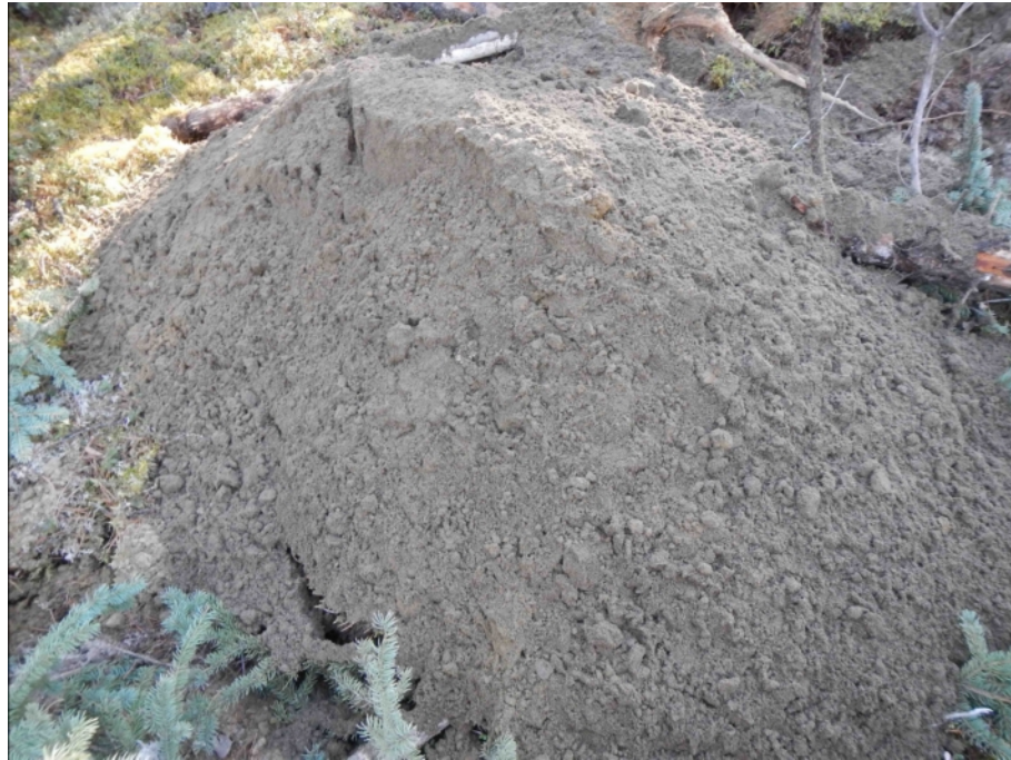
Figure 869-5328.1 Photo of Sample pile from 0.2m to 1.0m below ground level, from Test Pit 5328
