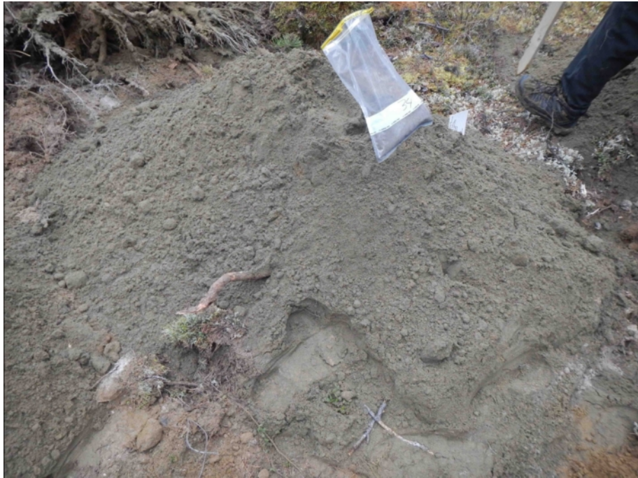
Figure 869-5331.2 Photo of Sample pile from 0.8m to 1.5m below ground level, from Test Pit 5331
