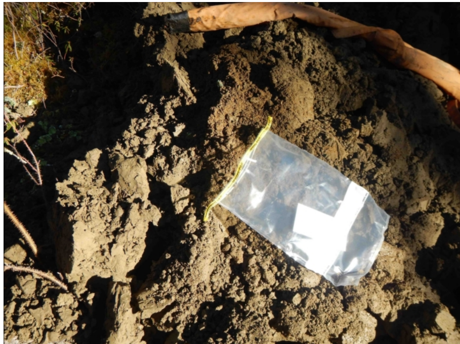
Figure 869-5326.2 Photo of Sample pile from 1.0m to 2.0m below ground level, from Test Pit 5326
