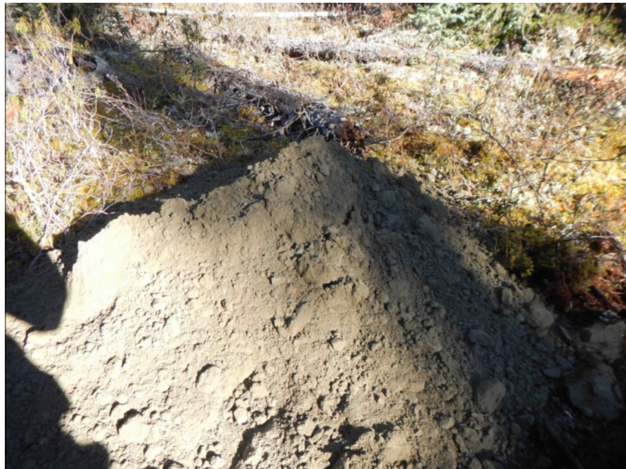
Figure 869-5322.4 Photo of Sample pile from 3.0m to 4.0m below ground level, from Test Pit 5322
