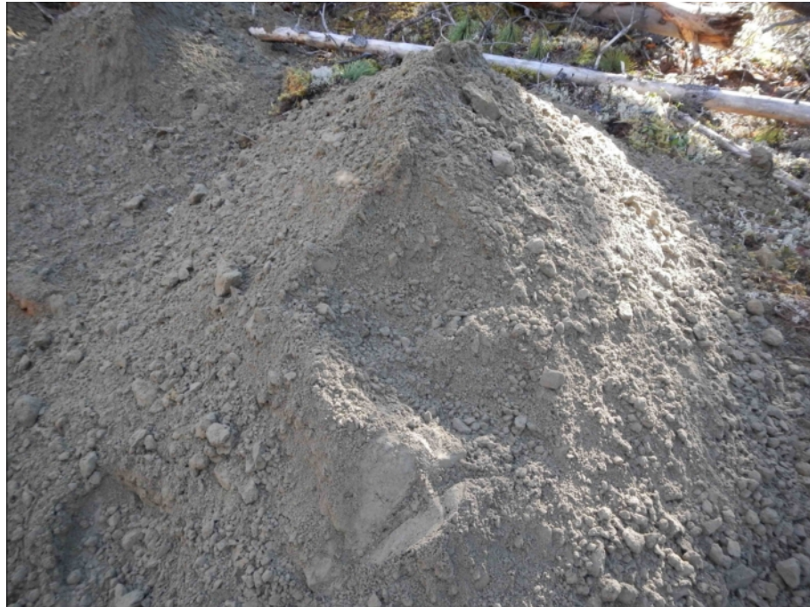
Figure 869-5324.1 Photo of Sample pile from 0.2m to 1.0m below ground level, from Test Pit 5324
