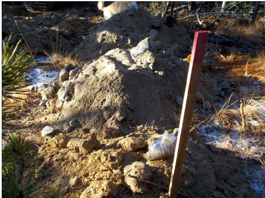
Figure 901-6585.2 Photo of sample piles from test pit 901-6585
