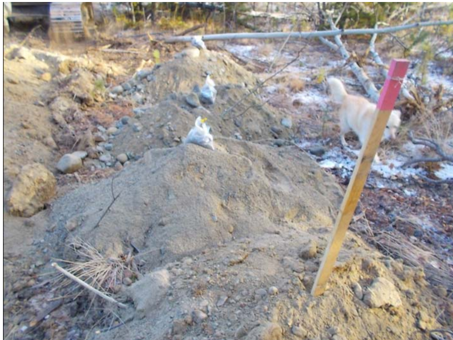
Figure 901-6582.2 Photo of sample piles from test pit 901-6582
