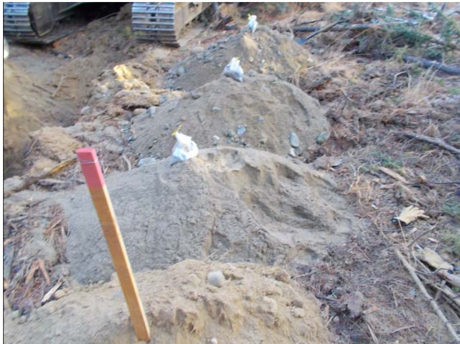
Figure 901-6580.2 Photo of sample piles from test pit 901-6580
