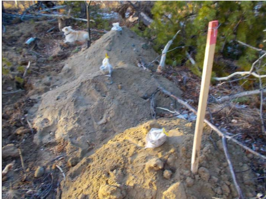
Figure 901-6591.2 Photo of sample piles from test pit 901-6591
