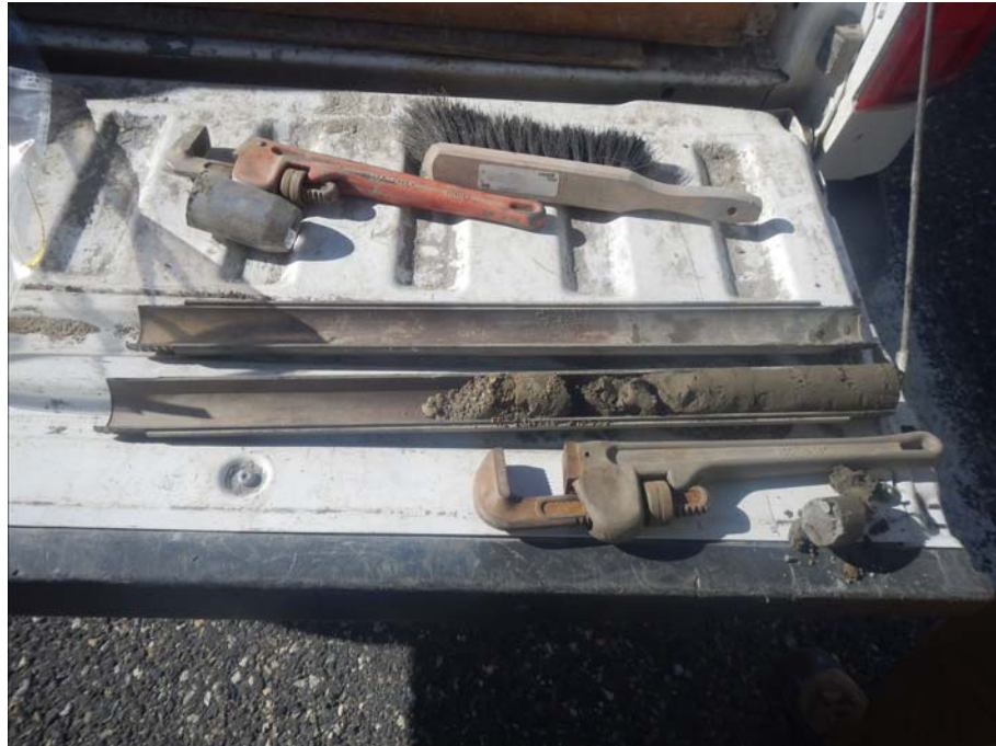
Figure 903-5711.2 SPT sample from 4.2 to 4.6m in BH903-5711
