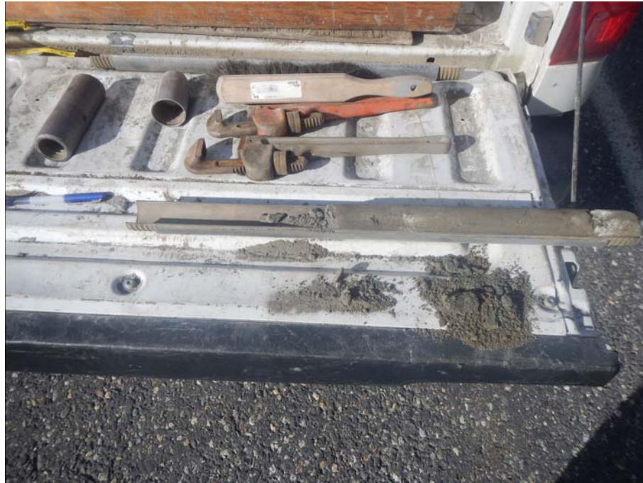
Figure 903-5710.1 SPT sample from 1.2 to 1.6m in BH903-5710
