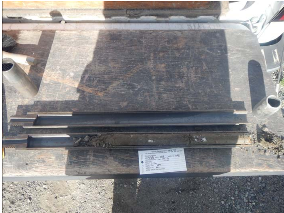
Figure 903-5716.2 SPT sample from 2.7 to 3.1m in BH903-5716
