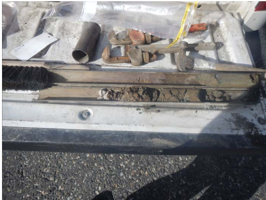
Figure 903-5710.2 SPT sample from 2.7 to 3.1m in BH903-5710
