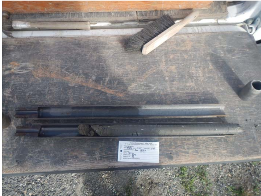
Figure 903-5715.3 SPT sample from 4.2 to 4.6m in BH903-5715
