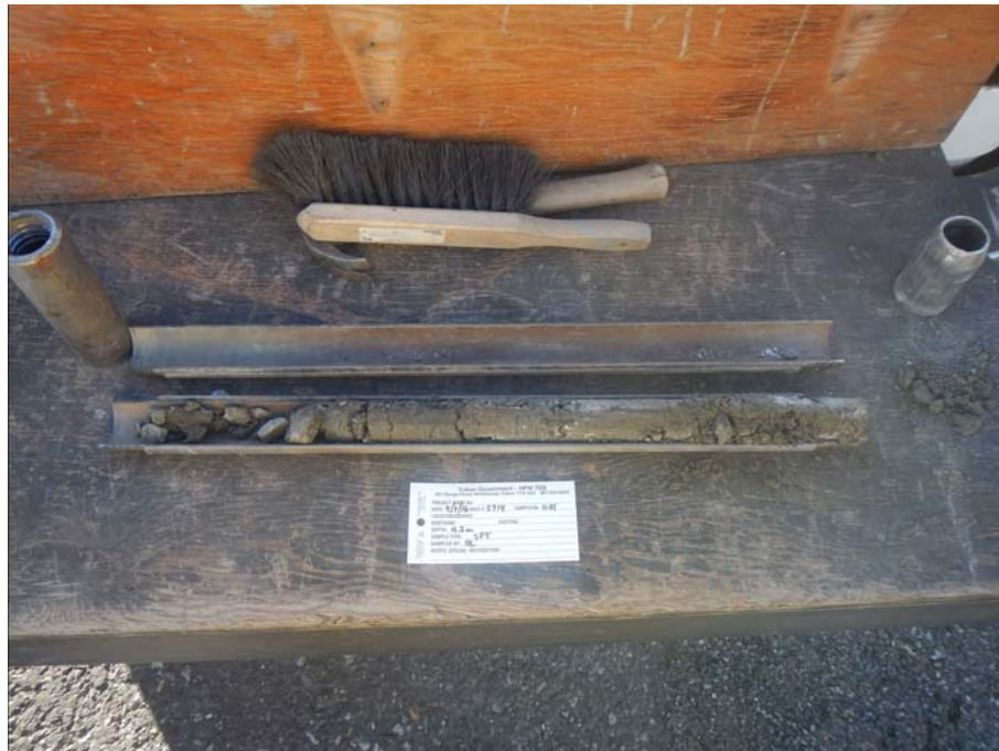
Figure 903-5714.2 SPT sample from 4.2 to 4.6m in BH903-5714
