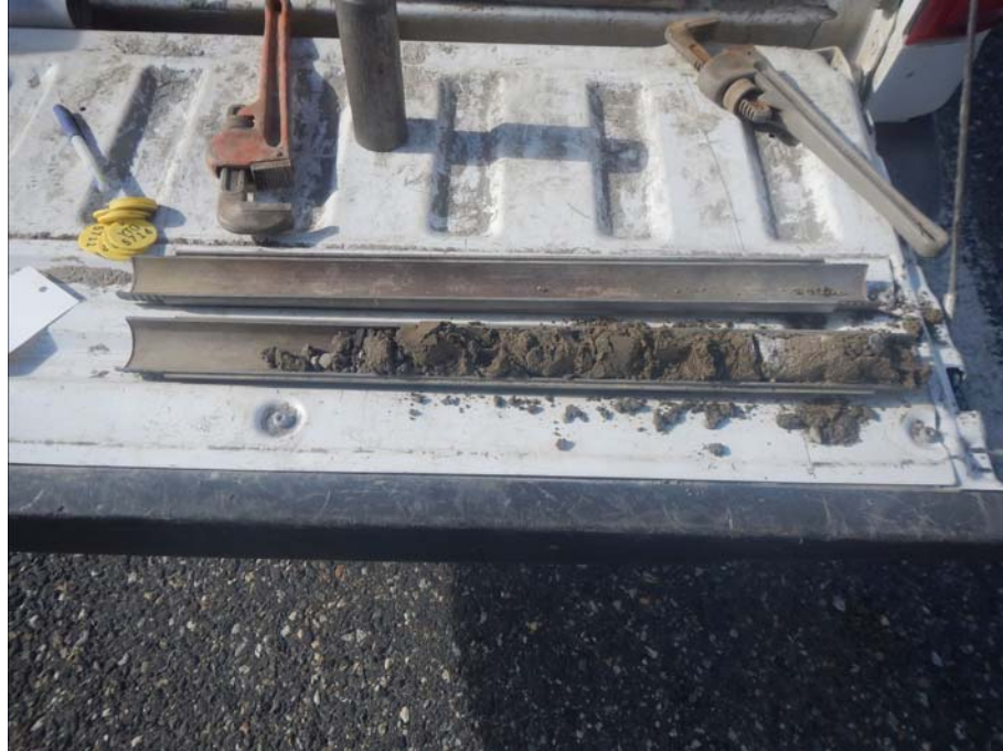
Figure 903-5711.1 SPT sample from 1.2 to 1.6m in BH903-5711
