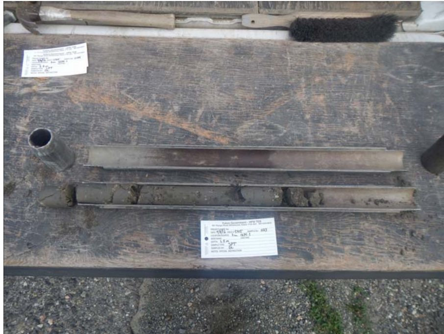
Figure 903-5715.1 SPT sample from 1.2 to 1.6m in BH903-5715
