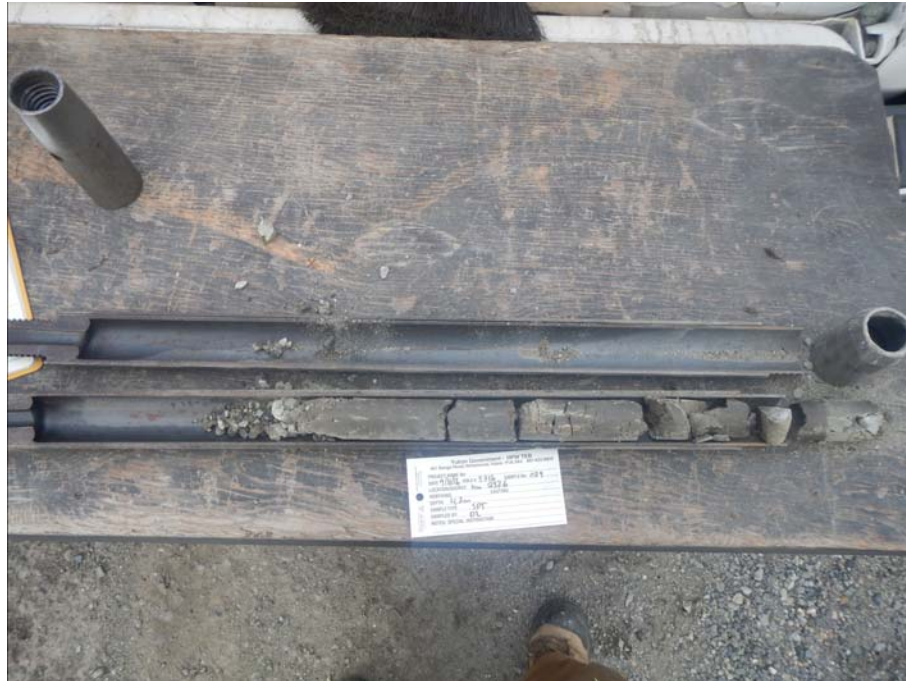
Figure 903-5716.3 SPT sample from 4.2 to 4.6m in BH903-5716
