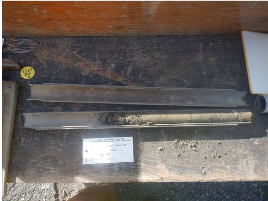
Figure 903-5713.1 SPT sample from 1.2 to 1.6m in BH903-5713
