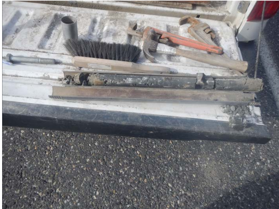
Figure 903-5710.3 SPT sample from 5.7 to 6.1m in BH903-5710
