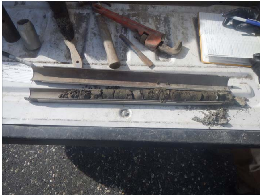
Figure 903-5712.1 SPT sample from 1.2 to 1.6m in BH903-5712
