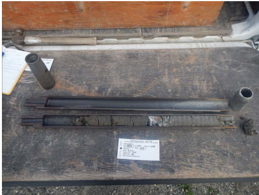
Figure 903-5715.2 SPT sample from 2.7 to 3.1m in BH903-5715
