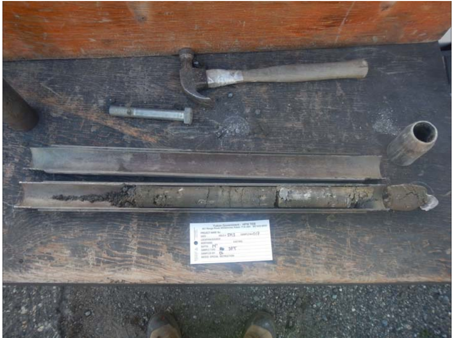
Figure 903-5713.3 SPT sample from 4.3 to 4.6m in BH903-5713
