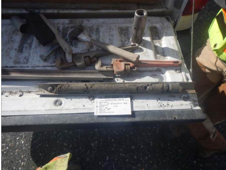
Figure 903-5712.3 SPT sample from 4.2 to 4.6m in BH903-5712
