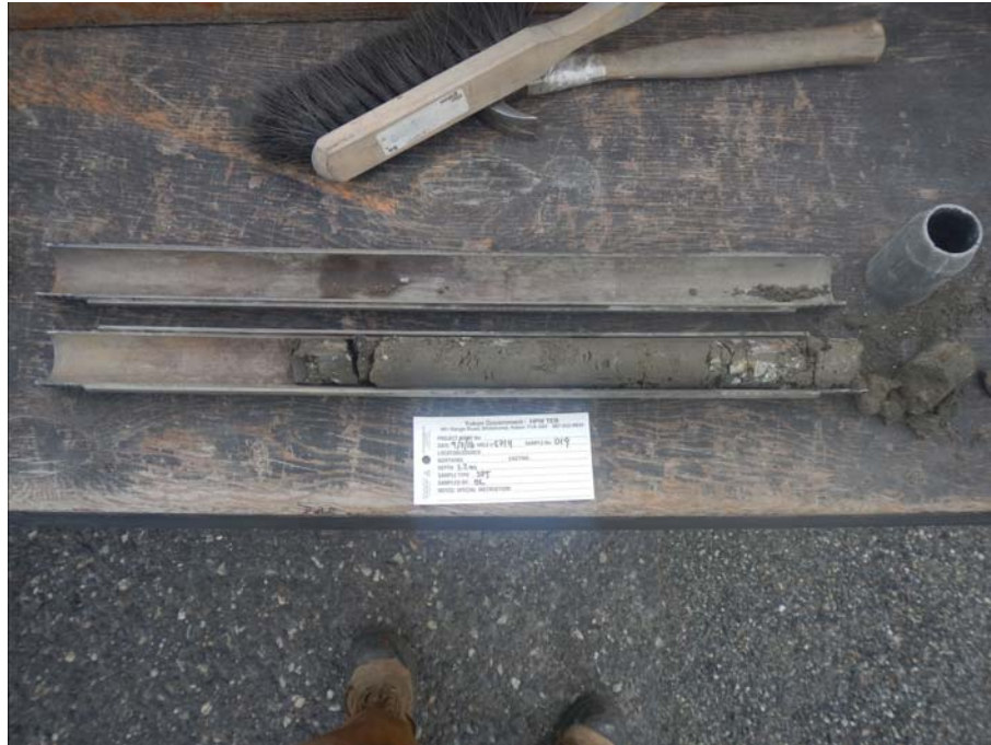
Figure 903-5714.1 SPT sample from 1.2 to 1.6m in BH903-5714
