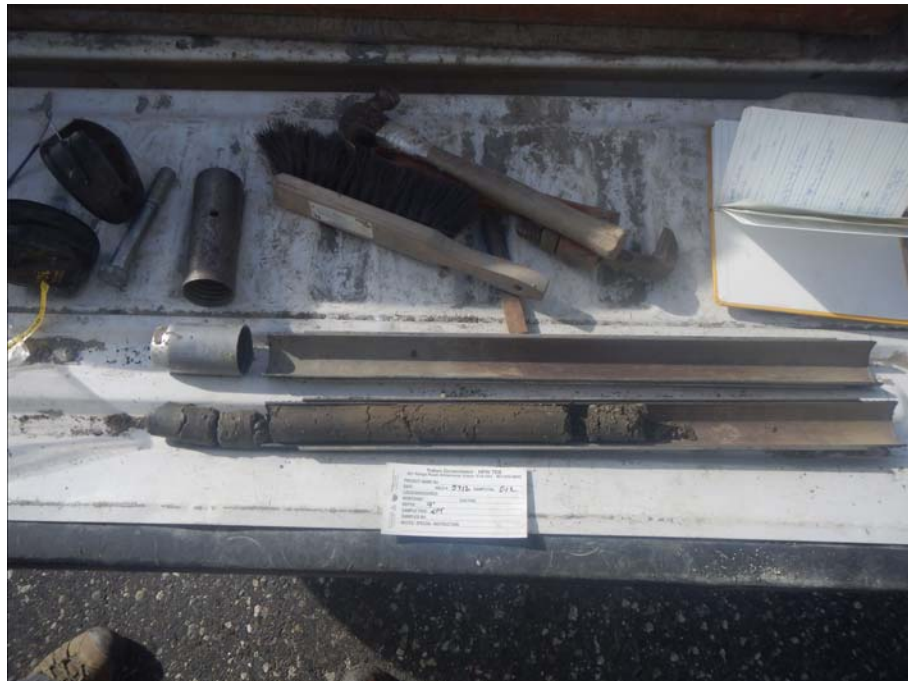
Figure 903-5712.2 SPT sample from 2.6 to 3m in BH903-5712
