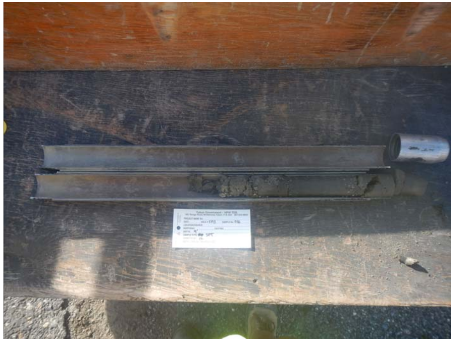
Figure 903-5713.2 SPT sample from 2.6 to 3.0m in BH903-5713
