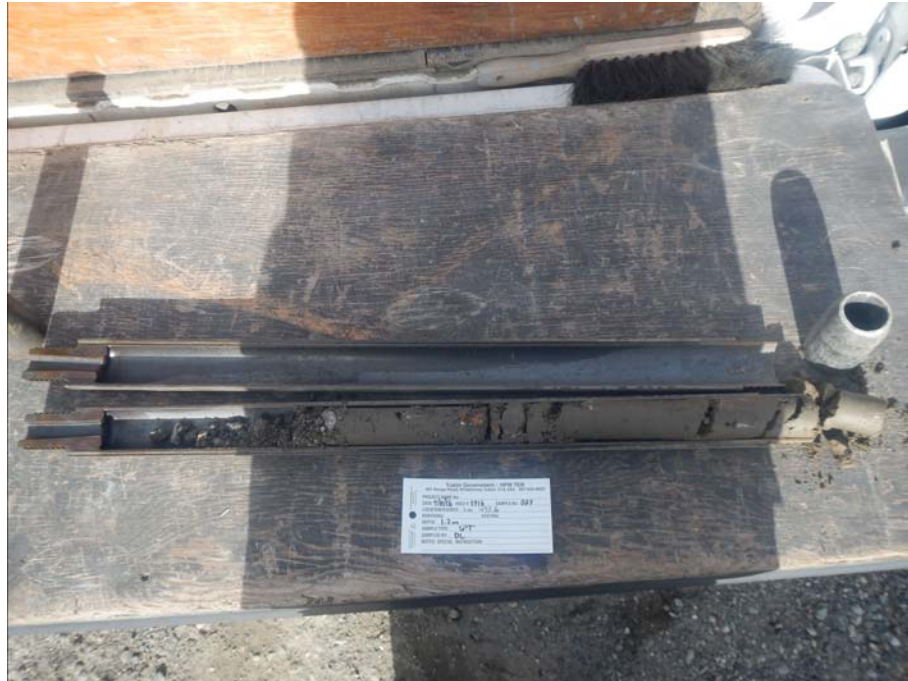
Figure 903-5716.1 SPT sample from 1.2 to 1.6m in BH903-5716
