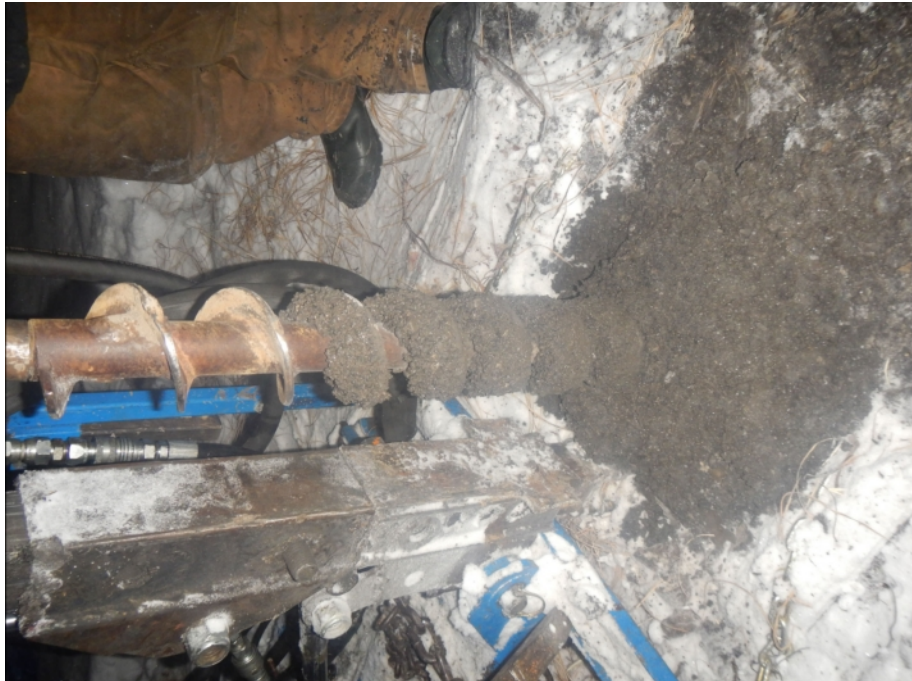
Figure 905-6605.2 Photo from borehole 905-6605 of material representative of soil strata between 3.0 and 4.5m.
