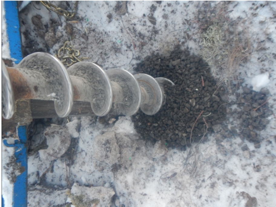
Figure 905-6595.1 Photo of drill cuttings coming up auger in borehole 904-6595 from 1.5 and 3.0m
