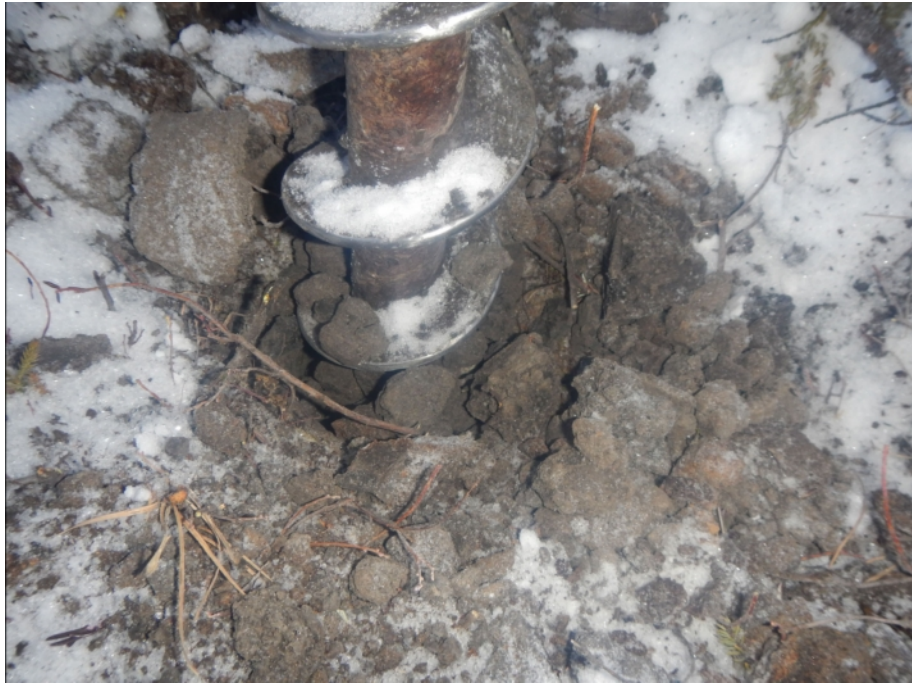
Figure 905-6606.1 Photo of drill cuttings from borehole 905-6606 representative of soil strata between 0 and 2.0m
