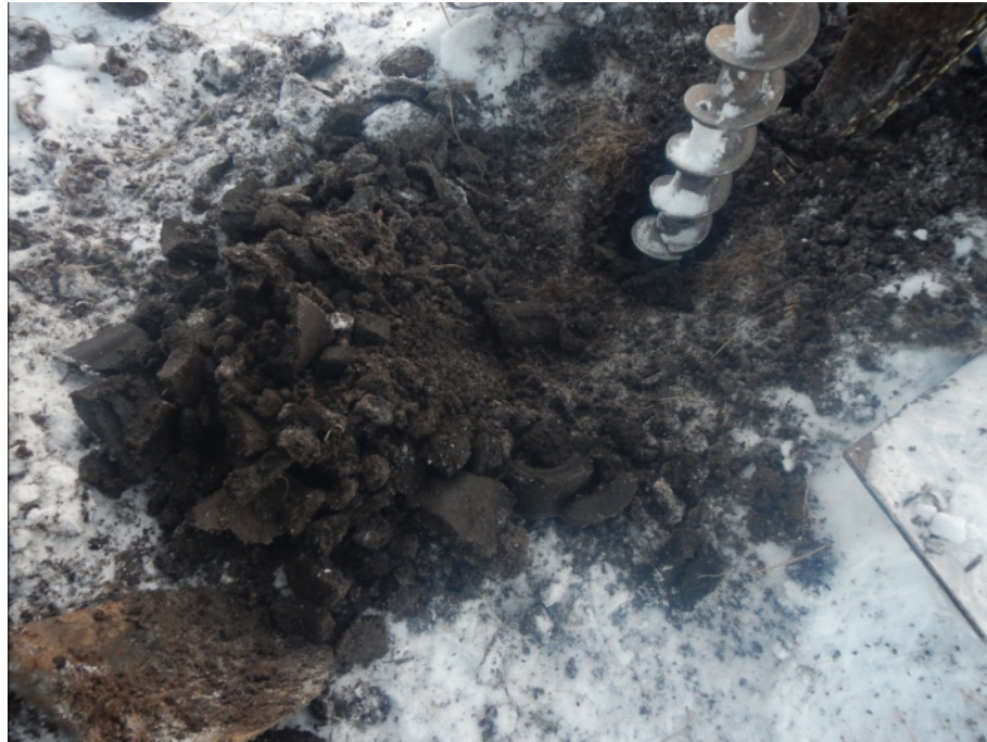
Figure 905-6604.1 Photo of auger cuttings from borehole 905-6603 representative of soil strata between 0 and 3.0m
