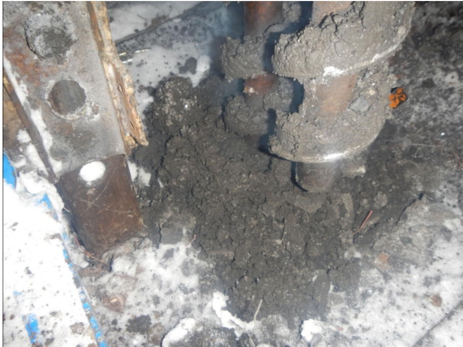
Figure 905-6607.2 Photo from borehole 905-6607 of material representative of soil strata between 3.7 and 4.5m
