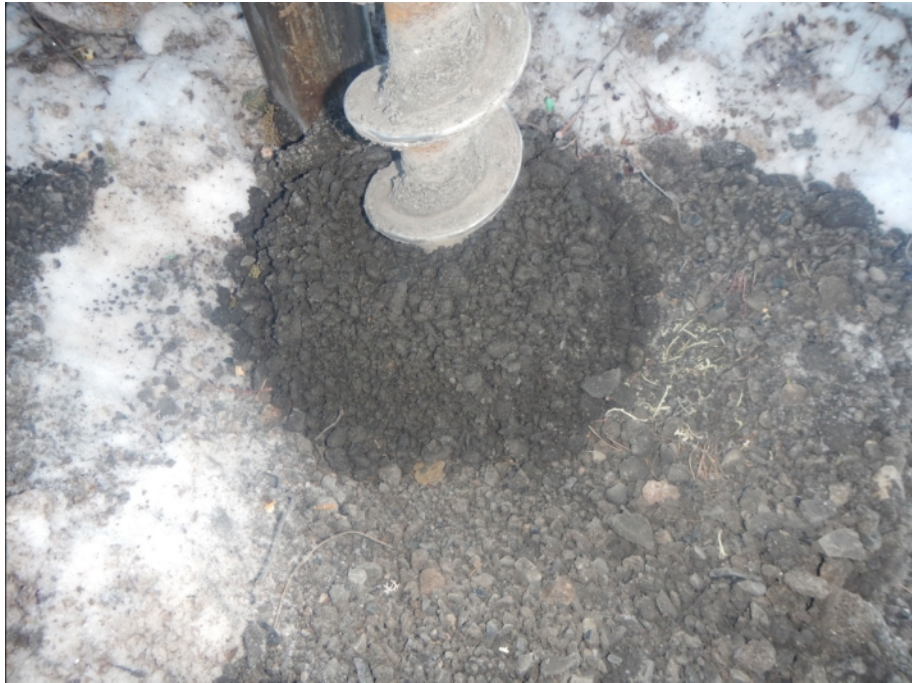
Figure 905-6595.2 Photo of drill cuttings coming up auger in borehole 904-6595 from 3.0 and 3.8m
