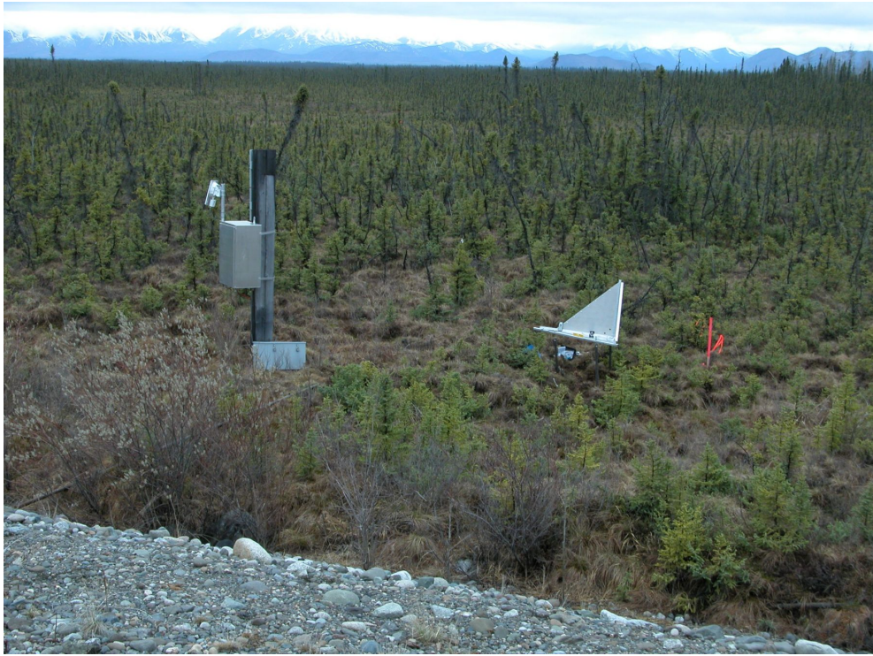
Figure 30 Radar reflector (to the right) and pre-existing data logger (to the left) used to monitor ground temperatures beneath and adjacent to the Alaska Highway at Beaver Creek, Site 2
