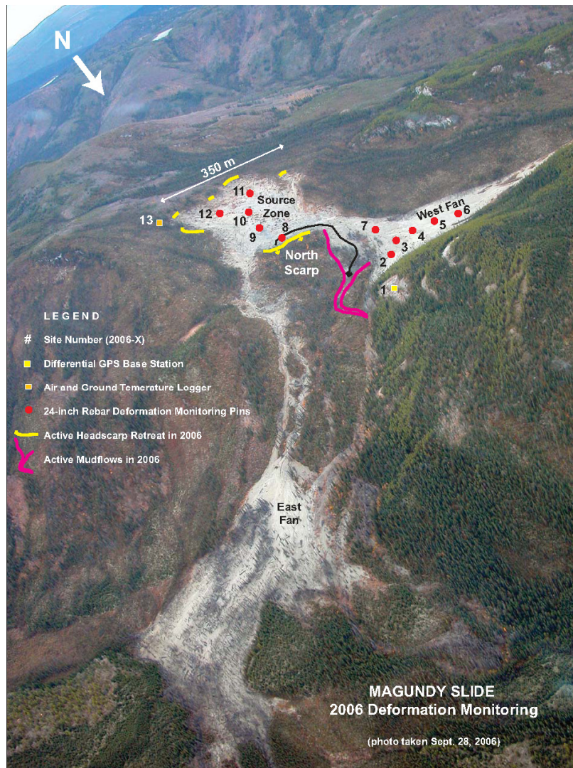
Figure 62 Deformation monitoring at the Magundy River Slide in 2006 (note that the horizon is rotated about 45° counter clockwise in this image)
