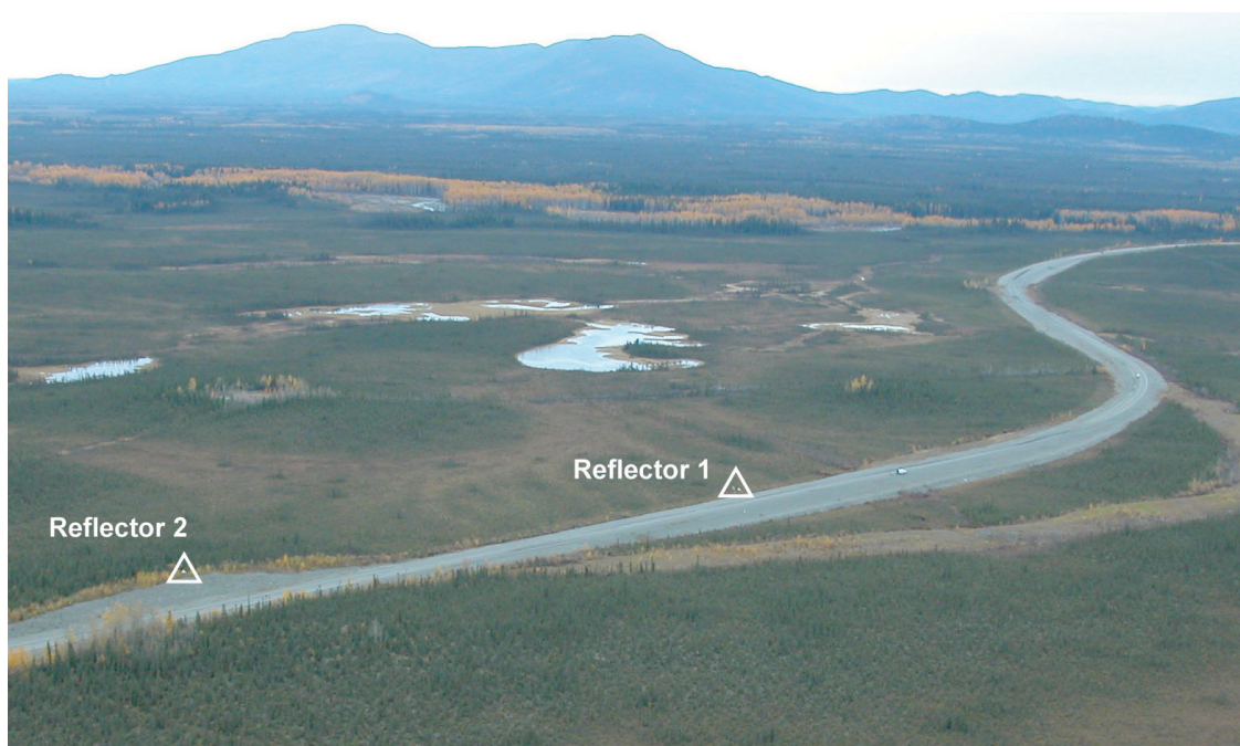
Figure 8 Oblique aerial photograph of the stretch of the Alaska Highway monitored at Beaver Creek Site 2. The distance between reflectors 1 and 2 is 370 m.
