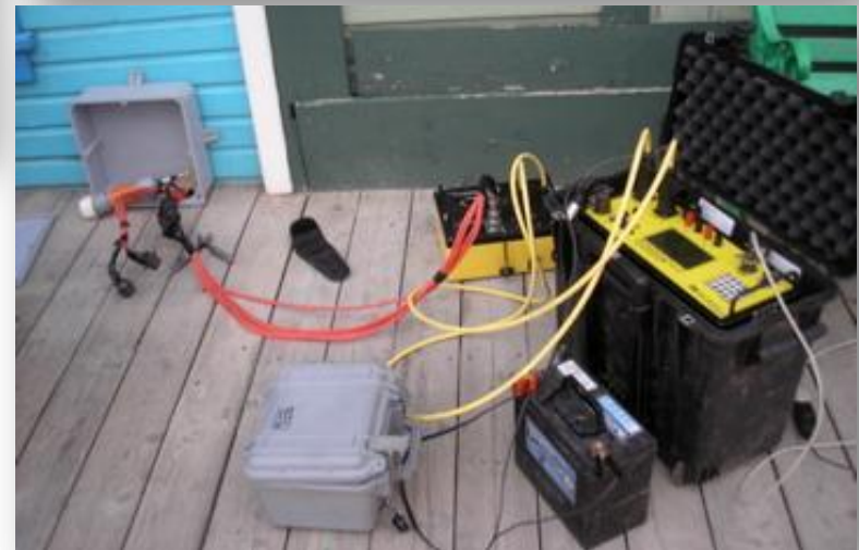
DC Resistivity Array Installation
