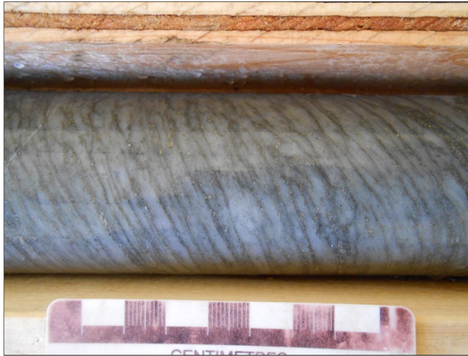
Felsic Lapilli Tuff- Light grey, strongly foliated, quartz sericite schist 1-2cm elongated aligned felsic lapilli
