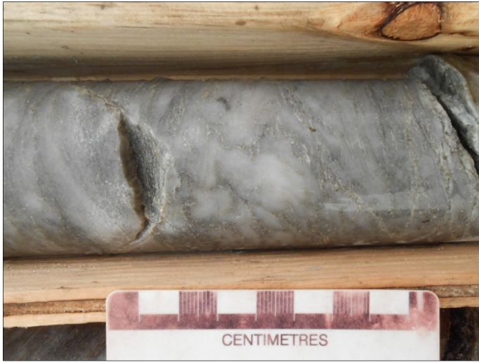
Massive Rhyolite - Light grey, massive to mottled quartz sericite schist. Possible flow banding and brecciation
