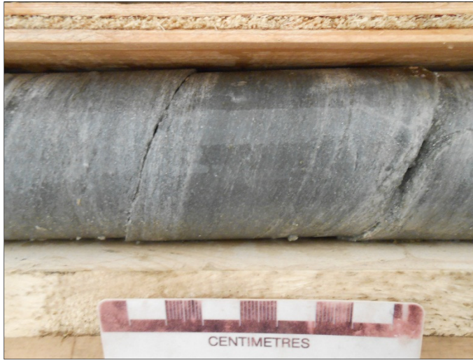
Felsic Ash Tuff - Fine grain, massive, weakly to moderately foliated quartz sericite schist
