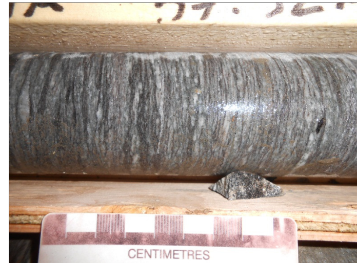
Siltstone/wacke - Med grey to med brown, strongly foliated, quartz biotite, chlorite schist
