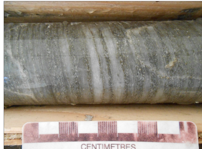
Felsic Lapilli Tuff- Light grey, strongly foliated, quartz sericite schist 1-2cm elongated aligned felsic lapilli
