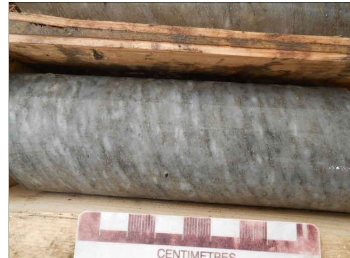
Feldspar Porphyry – Massive to foliated quartz feldspar sericite schist
