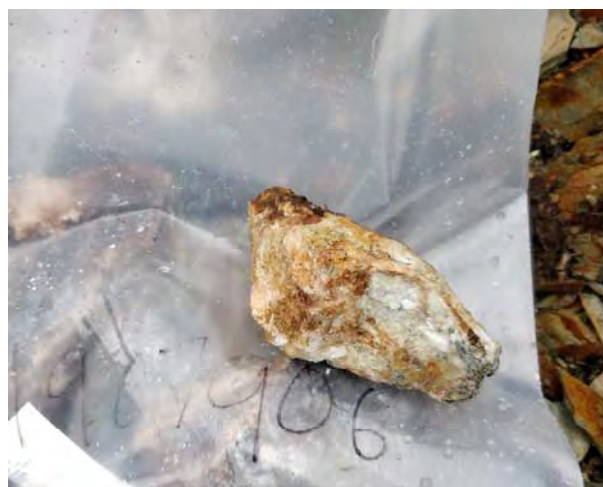
Figure 28: Sample 1907906 Quartz vein in Golden Culvert main showing striking 305°; 1% euhedral pyrite; assay of 13.38gpt Au.
