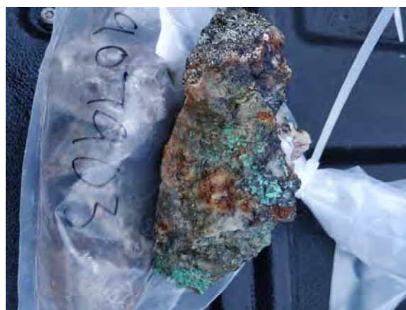
Figure 34: Sample 1907903 Green Dragon showing; quartz vein with disseminated chalcopyrite and malachite stain; assay of 6,575ppm Cu, 13,805ppb Ag.
