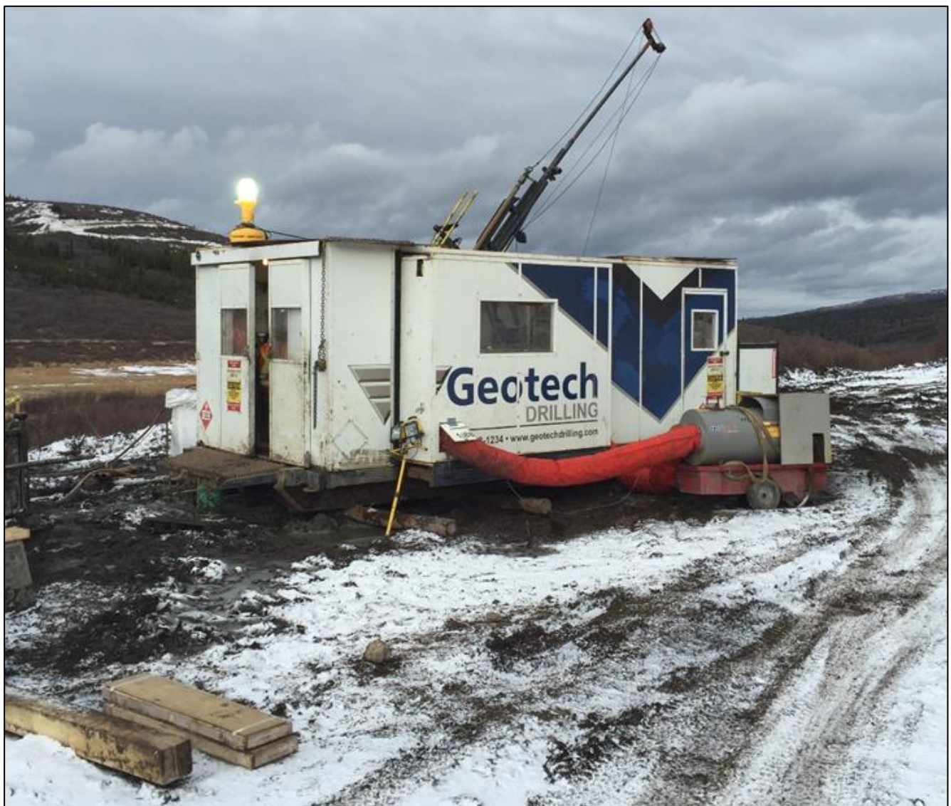
Figure 10-1: Geotech Drilling HC2000 drill rig at the ABM Zone on hole K15-291
