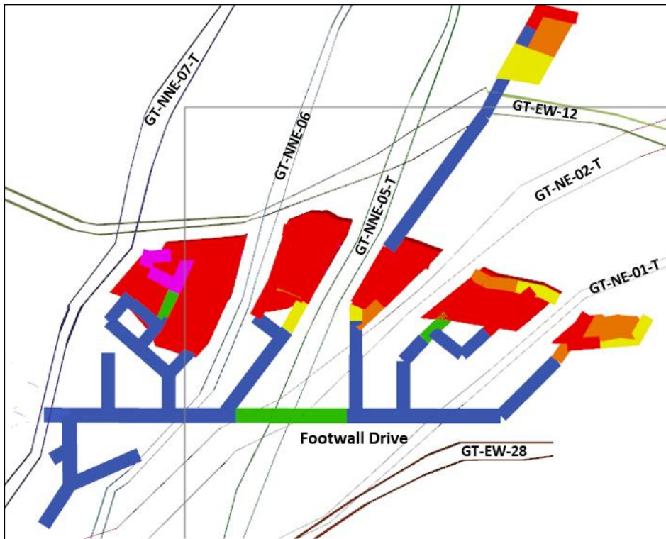
Figure 16-9: 1,225 mRL level showing main influencing faults
