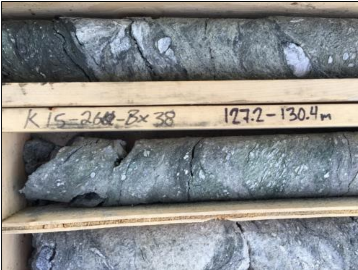
Figure 7-10: East Fault characterized by polyolithic fault breccia and minor gouge (K15-262 at approximately 127.2 m) Source: Hughes and Baknes, 2015
