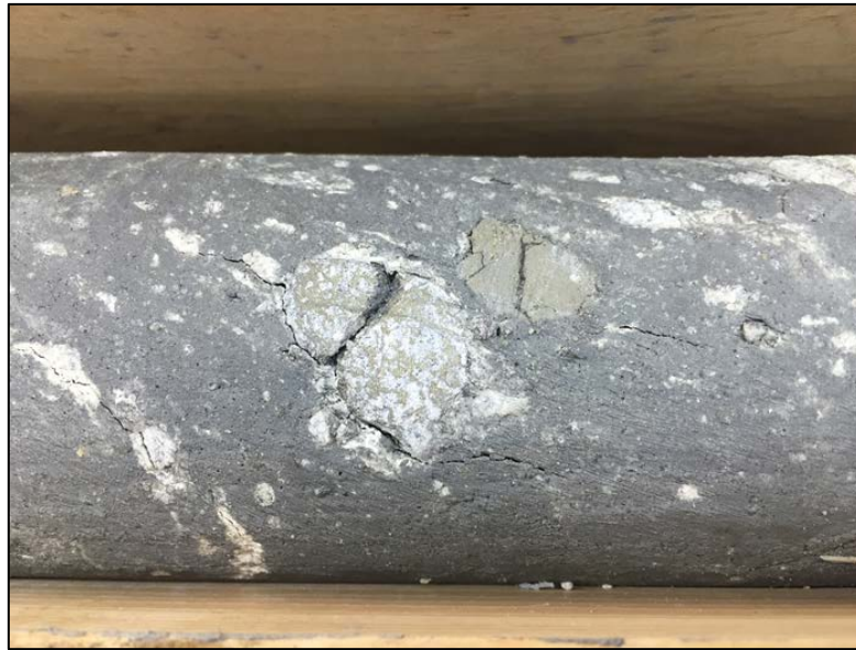
Figure 12: Angular to sub-rounded primary sulphide and sulphidised clasts within East Fault breccia (hole K15-292)
