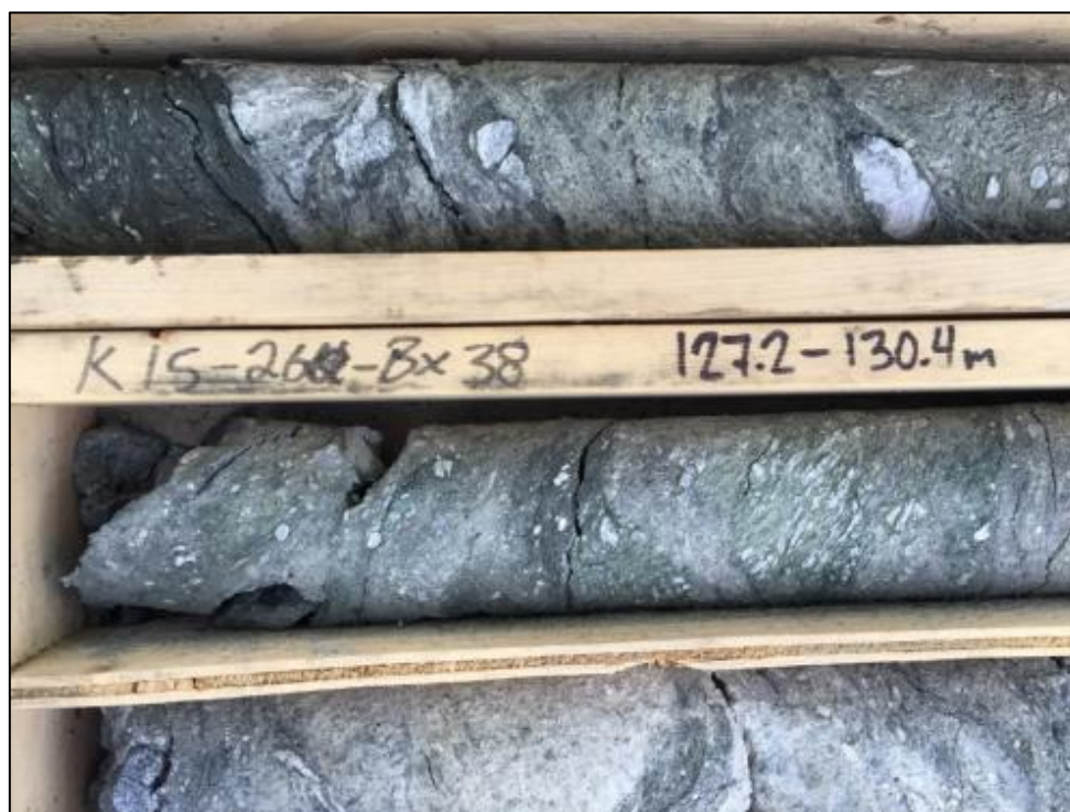
Figure 16: East Fault (D4) characterised by polyolithic fault breccia and minor gouge (K15-262 at ~ 127.2 m)
