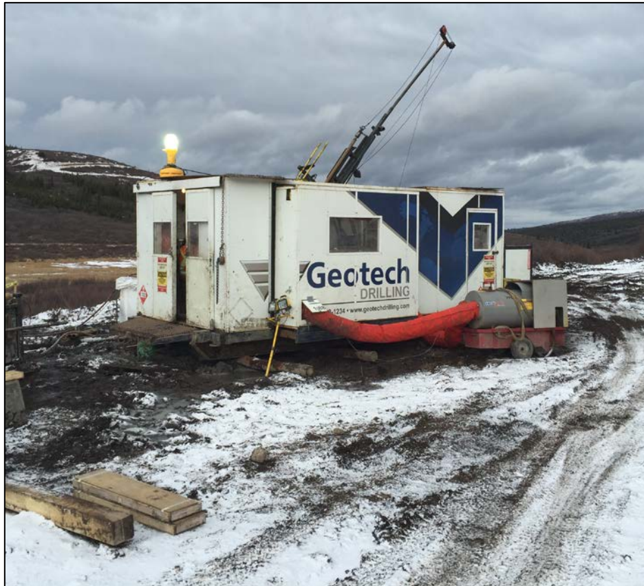
Figure 23: Geotech Drilling HC2000 drill rig at the ABM Zone on hole K15-291
