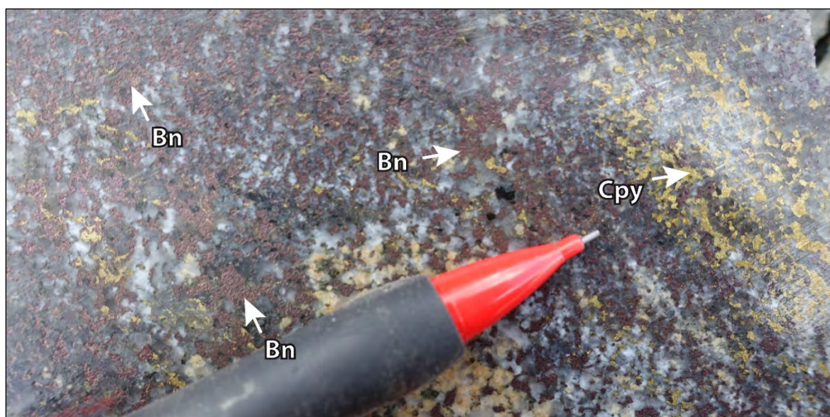
Figure 7-6: Net-textured Bornite-chalcopyrite in Migmatite, Minto Main Deposit
