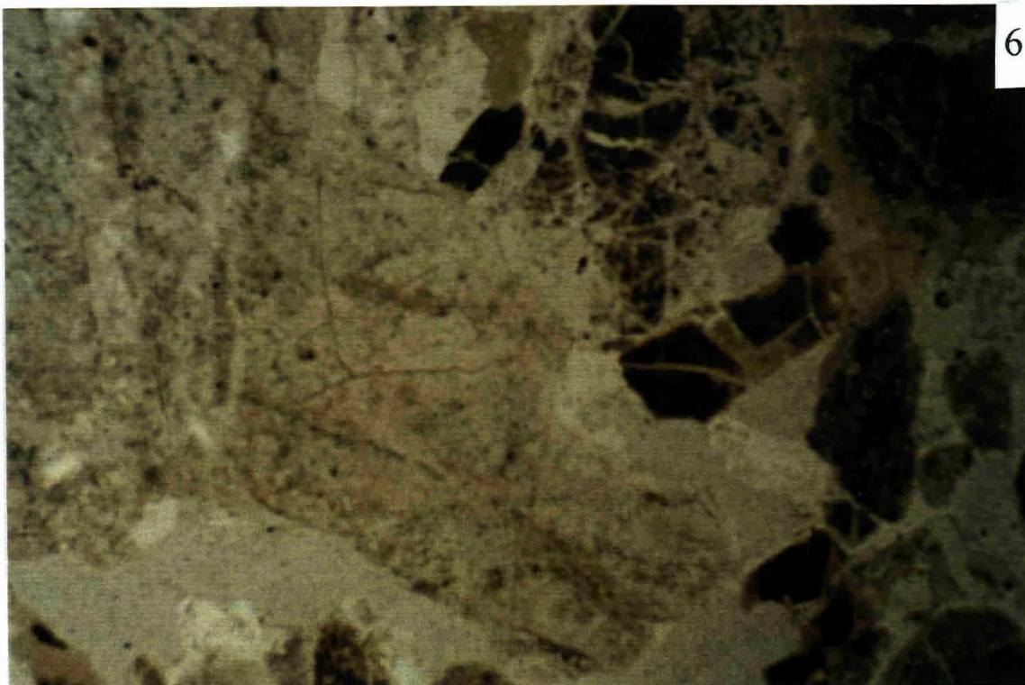
Birch B34 960.5' Jungle Creek Rock fragment, chert and quartz Conglomerate, buff-brown. 25x Volcanic rock fragments form large composite clasts. Quartz grains are polycrystalline, strained. Matrix of orthoquartzitic cement.
