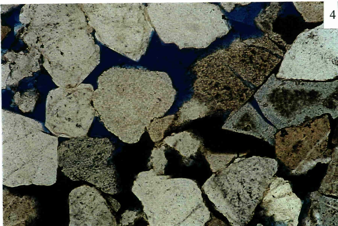
Birch B34 962.5' Jungle Creek Chert & Qtz arenite; f-med gr; some sutured grain boundaries; ~20%-30% primary porosity; quartz overgrowths; band detail shows diagenetic organic-rich clay or pyritic clay (?) 100x
