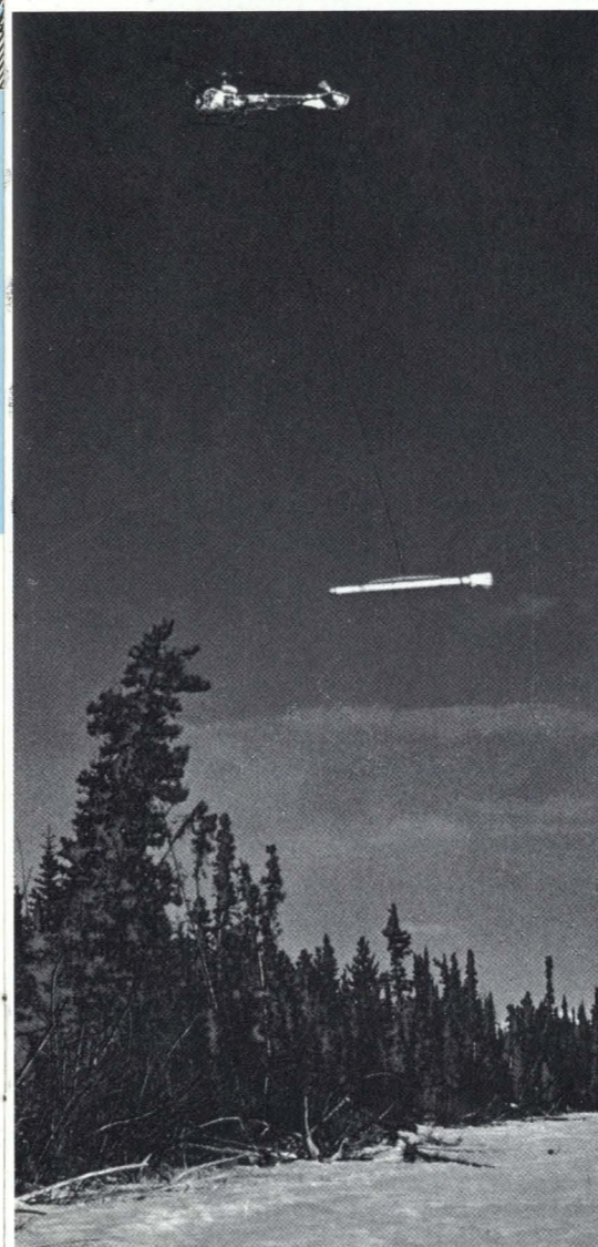
Helicopter-borne magnetic-electromagnetic survey used to detect anomalies.
