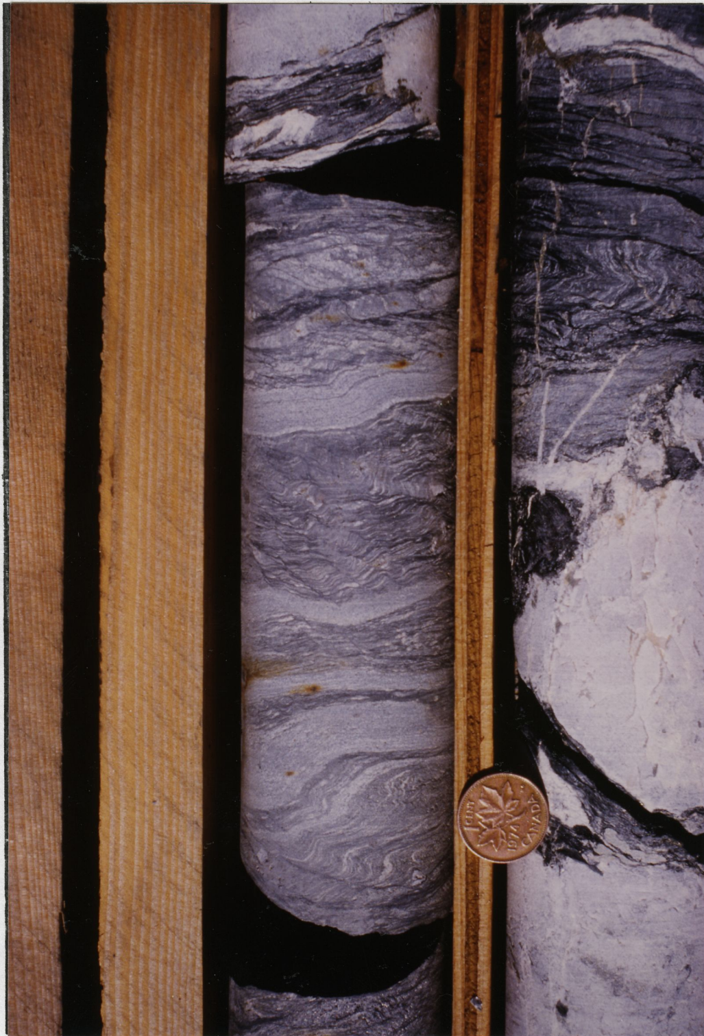
FIGURE 14. Photograph of drill core from the Grum deposit showing S_0 , S_1 , and S_2 in fine-grained graphitic schists.
