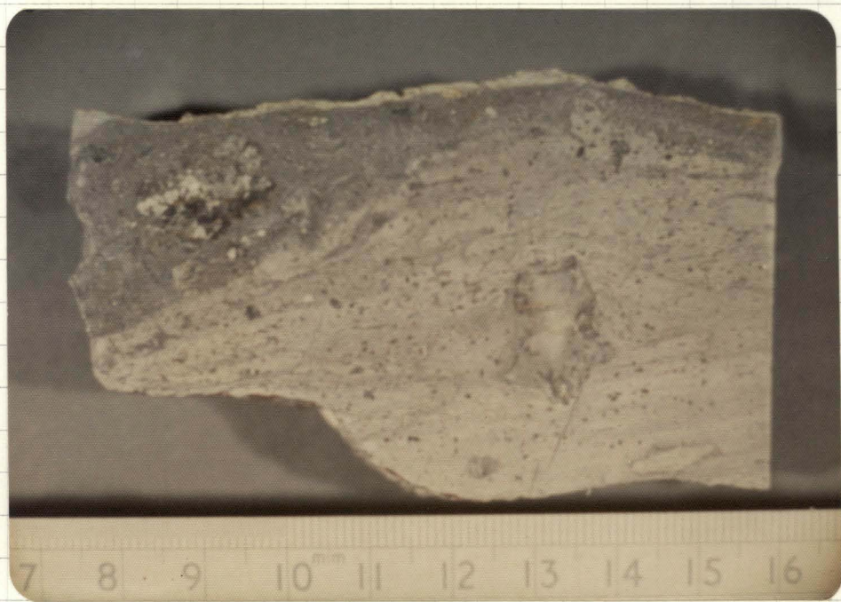
FIGURE 20 PYRRHOTITE SCHIST SAMPLE PLFO101, from which Figure 19 was produced. The upper surface is an early schistosity plane at the
