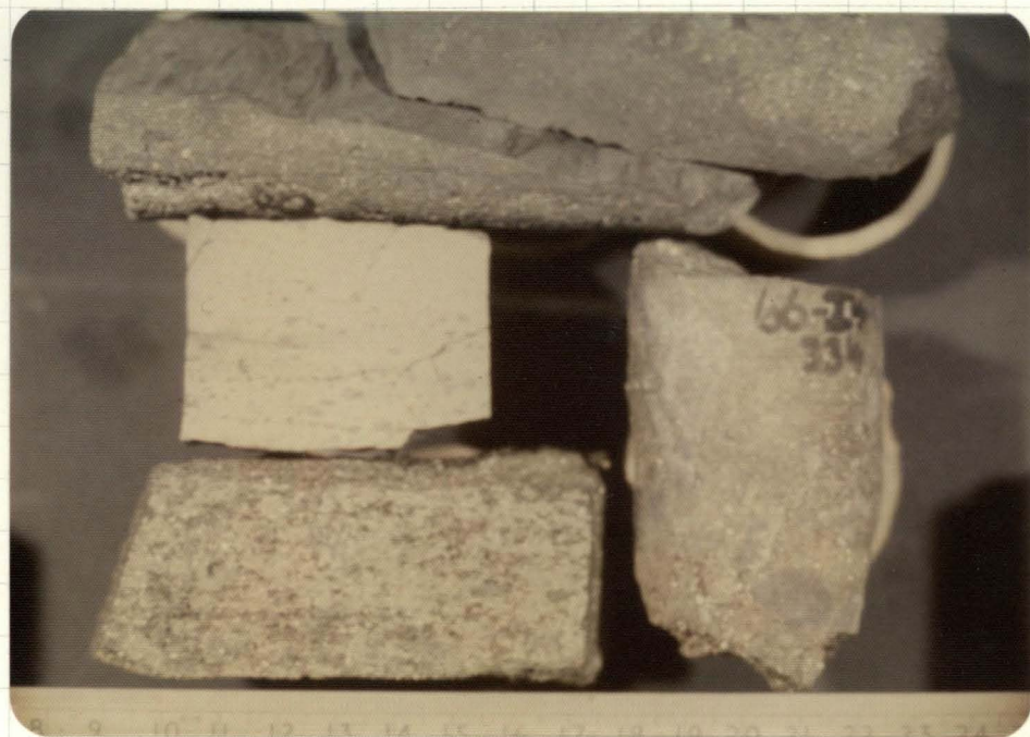
FIGURE 7 THE PYRITIC SULPHIDE FACIES Clockwise from the top: a) showing a fault polish surface with a 1 cm zone of triturated pyrite on either side b) showing an earlier breccia texture with fragments of quartzite and banded ore c) coarse, schistose and sandy with voids probably due to the
