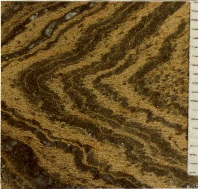
Plate 10: Bleached sericite phyllite interstratified with cherty bands. Scale in mm.
