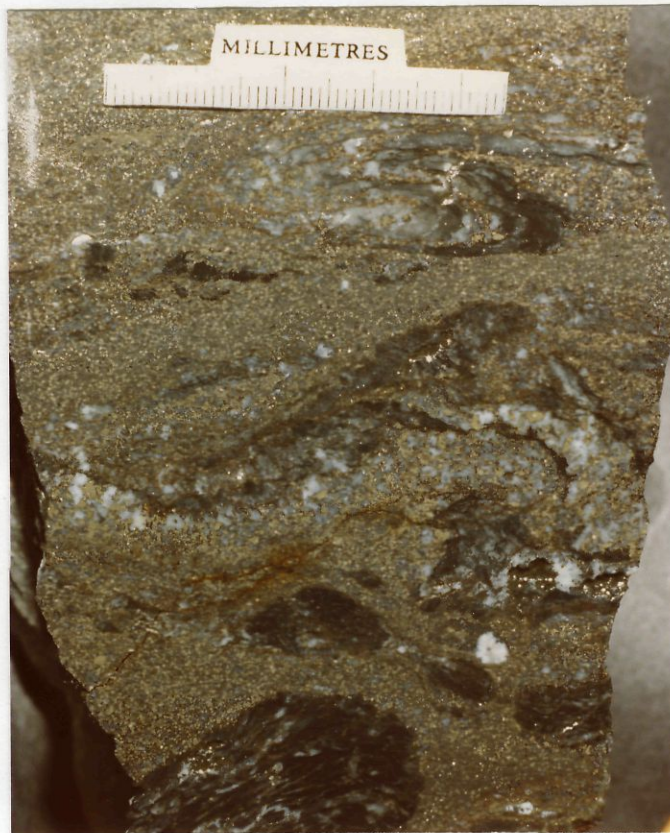
Plate 35 : Massive sulphide flowing around phyllite fragments.
