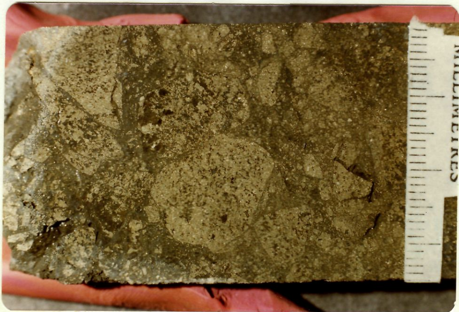
Plate 20: Brecciated massive sulphide (MX). Sulphide fragments are cemented by finer grain sulphides.
