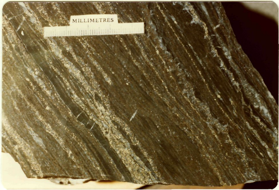
Plate 25: Banded quartz sulphide showing interlaminated sulphides and phyllite
