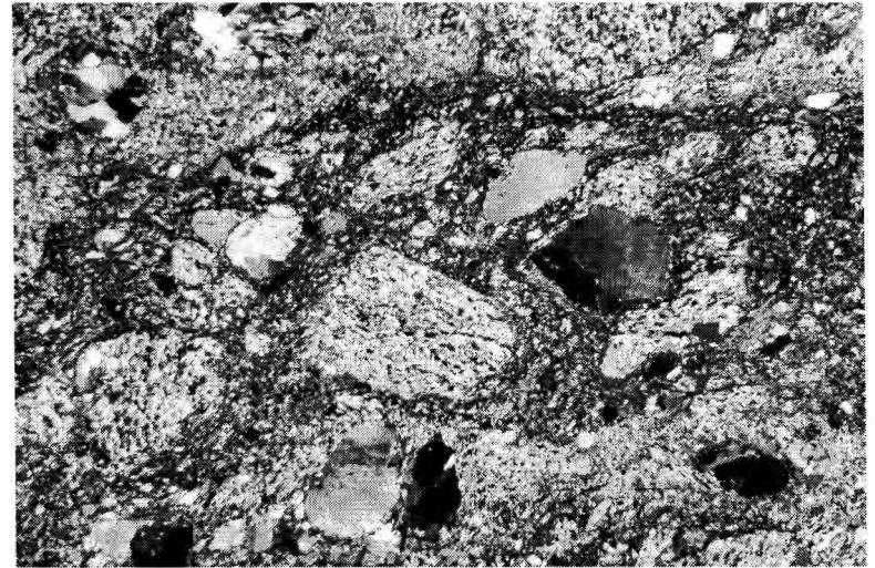
Plate 4. Quartz and sericite replacing elongated feldspar grains in felsic metavolcanic unit. Field of view = 7.2 mm.
