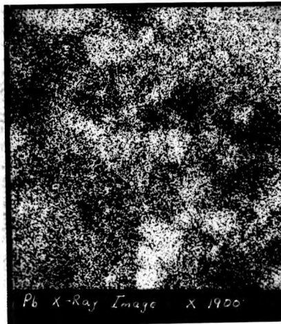
Fig. 2. Backscatter Electron Image and X-Ray Emission Images from the Second Selected Area of Lead Conc. Sample Jan. 1974.
