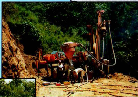
Reverse Circulation Drilling — Recio Vein, Guanacaste, Costa Rica.
