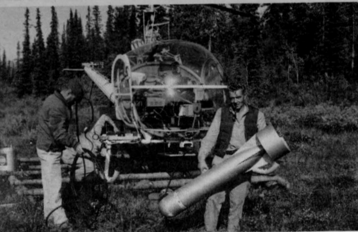
Starting Dynasty's aeromagnetic survey in the Vangorda area. A Hiller 12E helicopter, chartered from Klondike Helicopters, is being installed with $65,000 worth of electronic gear by Harold Sanian of Hunting Surveys while pilot Jim Burke unwinds the cable and prospector director Alan Kulan holds the "Bird". This work, followed by preliminary drilling led to the major drilling program.
