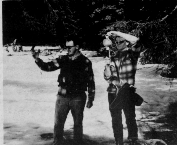
Ground magnetometer survey was made on Swim Lake in May 1964. Here Andy Harman is setting a compass bearing across the ice while Bill Barclay is taking a magnetometer reading. Dynasty's first target, the SEA anomaly, was later outlined by this survey.
