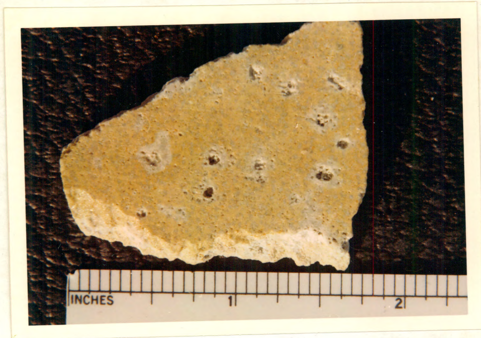
Plate 19. Sulphides are completely leached from rock. Transported \text{Fe}^{++} has precipitated as jarosite, staining rock.
