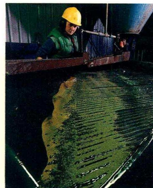
Tons of rock were mined and crushed to yield the gold on this shaker table
