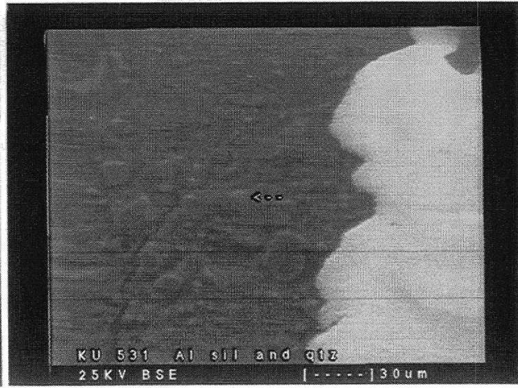
KU 531 orthocl, allophane 25KV BSE |-----| 30um ALLOPHANE AND ORTHOCLASE IN GOLD.
