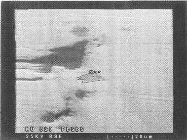
KU 520 Bi and Bi oxides 25KV BSE |-----| 20um BISMUTH OXIDES IN GOLD.
