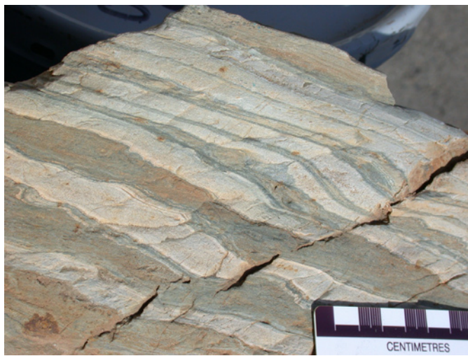
Figure 21. Contact hornfelsed Vangorda formation phyllite adjacent to massive greenstone lens. Light bands are quartz-calcite siltstone and dark bands are greenish muscovite-quartz-chlorite phyllite. Field station 98LP026 on Swim Lake road.
