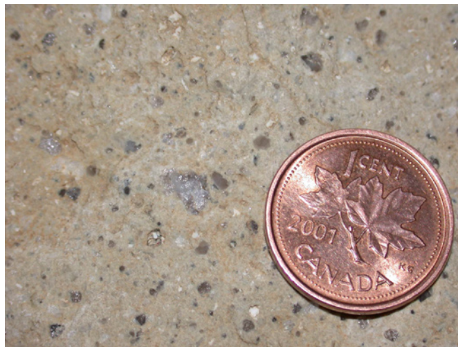
Figure 58. Eocene quartz-feldspar porphyry. Smokey quartz and small white feldspar phenocrysts. Sample from northeast wall of Faro open pit. Penny is 1.9 cm across.
