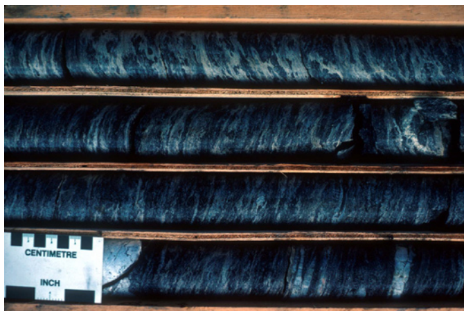
Figure 7. Mount Mye formation. NQ-size core. Biotite-andalusite clots and clusters within matrix of biotite-muscovite phyllite transitional to schist. Dominant foliation is closely spaced crenulation cleavage. Drill hole 84F-28.
