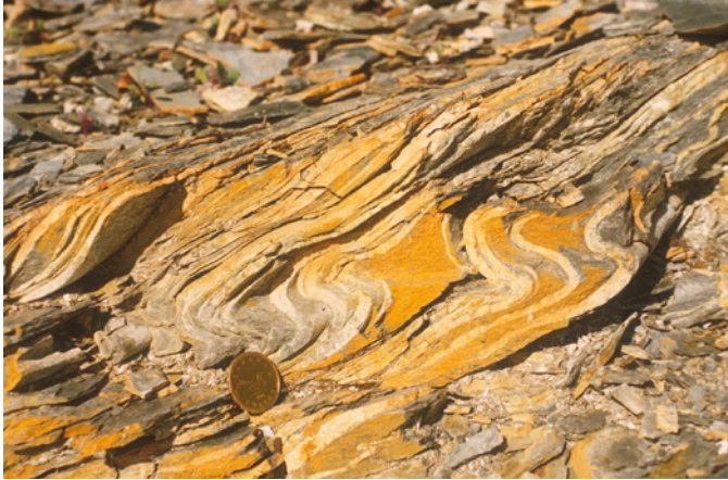
Figure 14. Vangorda formation phyllite. Light grey to white quartz-calcite siltstone interbeds in silvery grey, noncalcareous to slightly calcareous muscovite-chlorite phyllite. Coin is 2.7 cm wide.
