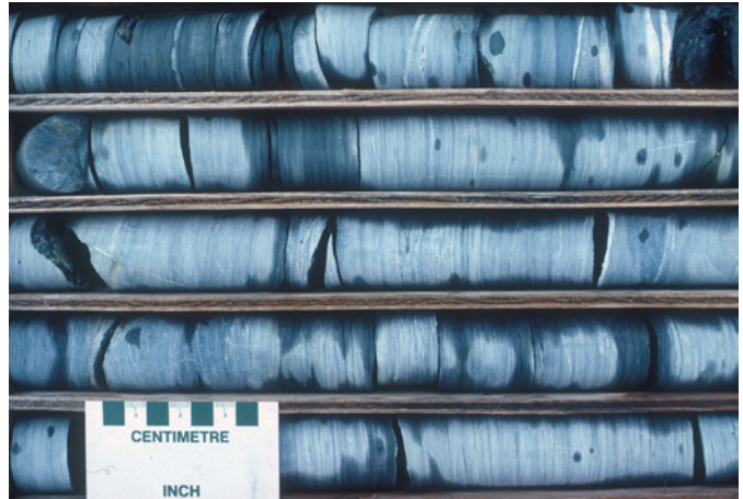
Figure 5. Mount Mye formation phyllite. BQ-size core. Core breaks on finely spaced crenulation cleavage which forms the dominant foliation. Note minor colour variations are transposed subparallel to dominant foliation. Drill hole CNR76-01, 426 ft – 449 ft (130 m – 137 m).
