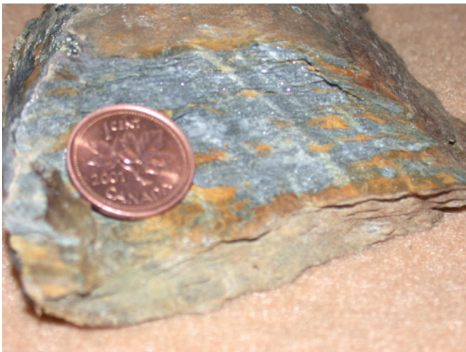
Figure 4. Mount Mye formation phyllite. Weathering consists of a brownish coating. Bedding is visible progressing from top to bottom of photo near the centre. Canadian penny is 1.9 cm across.
