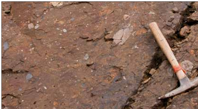
Figure 5. Pebbly mudstone of the Toobally Formation, with slaty cleavage, dipping to the left (west). Hammer handle is 33 cm long. West of upper Toobally Lake, station 03LP006.
