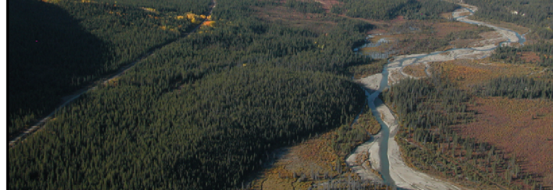
Figure 2. Large active alluvial fans spill into the Wheaton River valley from tributary streams. In this photograph at the base of Tally-Ho Mountain a debris flow hazard exists where the Wheaton River Road traverses the fan (see arrow). These surficial deposits are a good source of aggregate.
